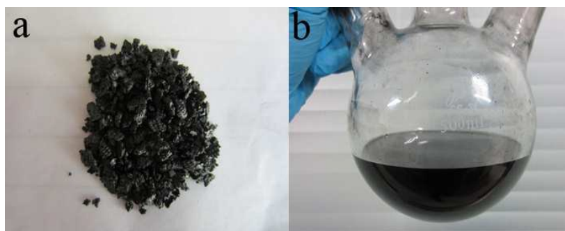
Fig. 1. The dispersion process of lump CNTs-COOH in 1-chlorobutane and N-methylimidazole system: (a) the lump CNTs-COOH; (b) the [Bmim]Cl/CNT-COOH system.
