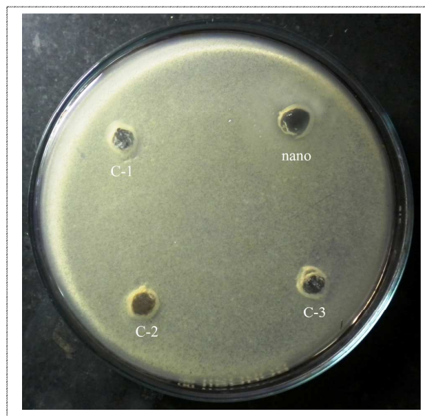
Figure 7. Antibacterial study on different test samples by agar diffusion method in a petri dish. C-1 contained GG + PVA + AgNO 3 , C-2 contained PVA + AgNO 3 , C-3 contained GG + AgNO 3 , nano contained AgNPs 70/30/6.1 at a concentration of 1mg/ml. Image clearly showed an inhibitory zone of various diameters around each cavity. Antibacterial study was initiated using 3 days old AgNPs 70/30/6.1 .
