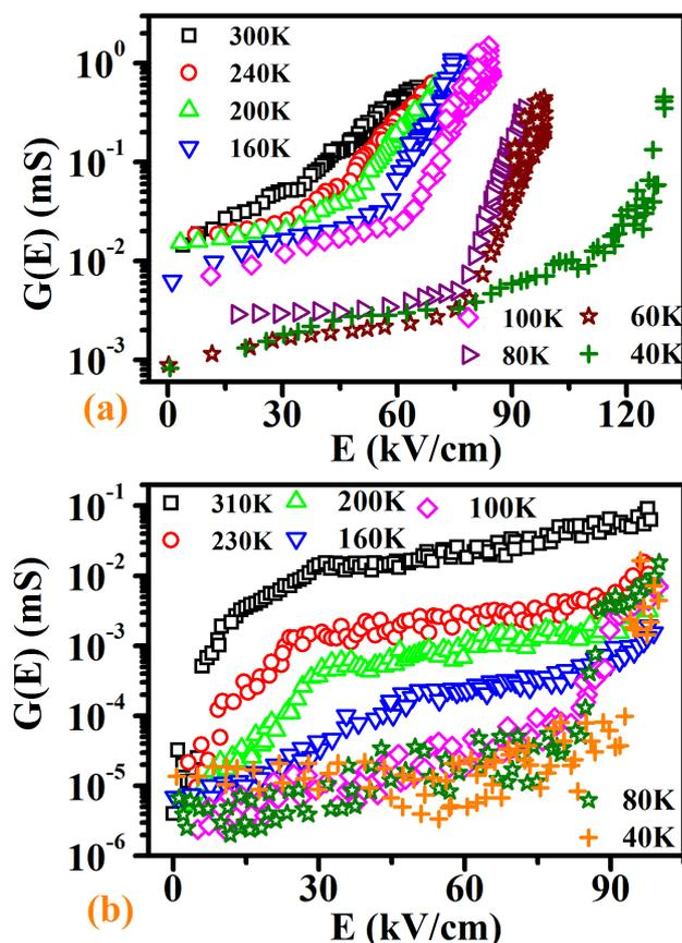
FIG. 4: (Color online) Bias dependent conductance  $G=dI/dV$  of NWs grown (a) with and (b) without field. The value of  $G$  has been scaled by number of wires to make  $G$  the conductance of a single NW.
