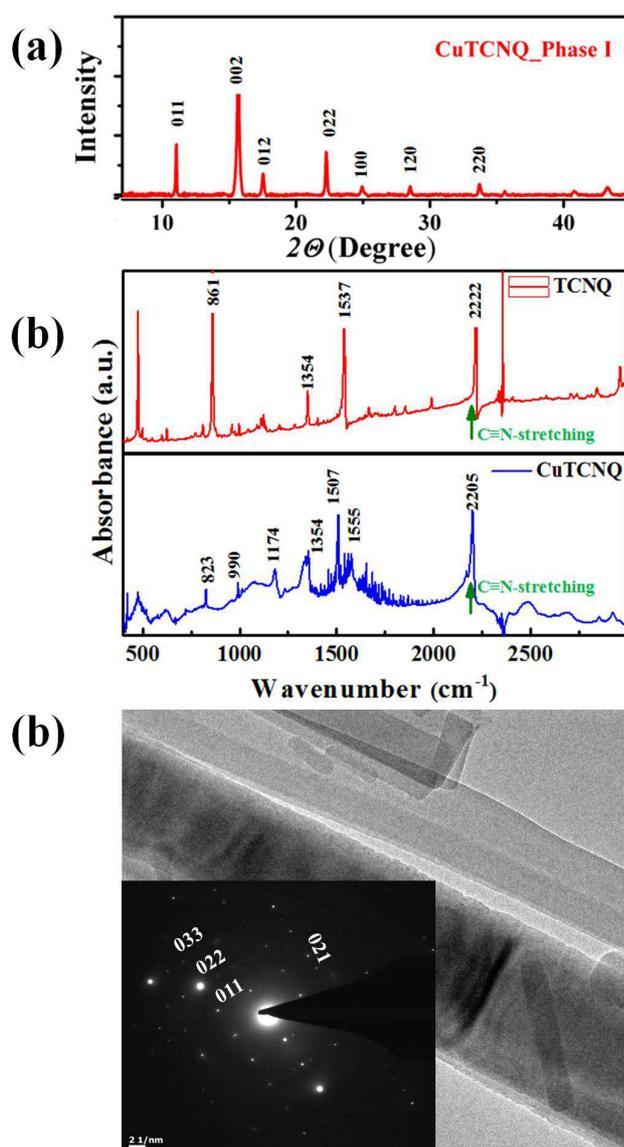
FIG. 2: (Color online)(a) X-ray diffraction patterns of PVD grown NWs. The indexing is as per ICDD data base. (b) FTIR spectra of TCNQ and Cu:TCNQ. Shift in  $-CN-$  stretching mode gives the degree of charge transfer  $Z$  estimated from ref. [20]. (c) TEM image of Cu:TCNQ NW dispersed on a TEM grid. (Inset) Selected area electron diffraction (SAED) pattern of the NW to show its single crystalline nature.
