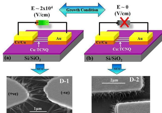
FIG. 1: Schematic of the device for inplane growth of Cu:TCNQ NW within prefabricated pads (a) with and (b) without field. SEM images of Cu:TCNQ NWs corresponding to the growth conditions are represented by arrows.
