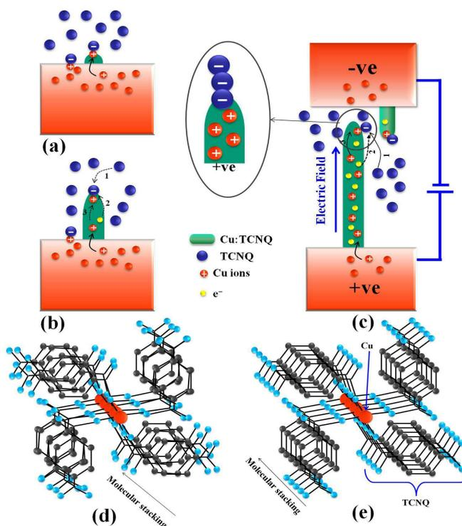
FIG. 8: (Color online) Schematic of Cu:TCNQ NW growth under externally applied field. (a) Nucleation of the ions, (b) NW growth and (c) accelerated nucleation process under field. Stacking of the Cu:TCNQ molecules during growth (d) without field and (e) with field. Field growth NW are having better  $\pi - \pi$  stacking of the TCNQ molecules.
