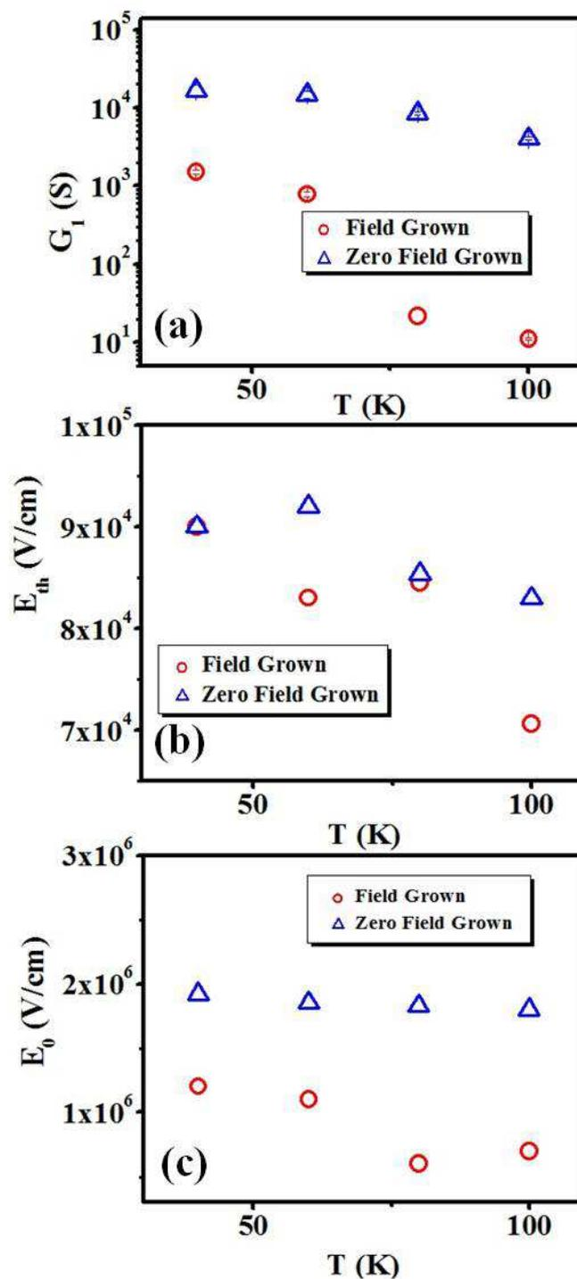
FIG. 7: (Color online) Temperature dependence of the parameters (a)  $G_1$ , (b)  $E_{th}$  and (c)  $E_0$  as obtained from the fit to modified Zener tunneling relation as shown in Fig. 5.
