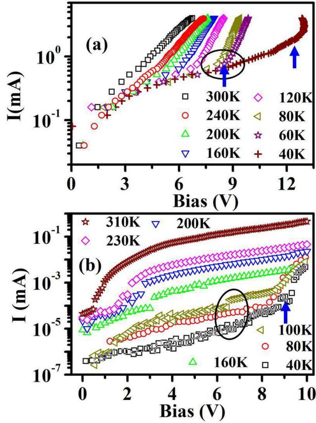
FIG. 3: (Color online) I-V data at different temperatures of NWs grown (a) with field,  $E \sim 2 \times 10^4$  V/cm and (b) without field,  $E \sim 0$  V/cm. The  $V_{th}$  for temperatures  $T < 100$  are marked by circles and arrows.
