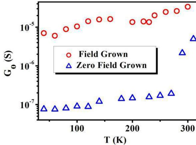
FIG. 6: (Color online) Temperature dependence of the linear conductance  $G_0$  (calculated from the slope of linear region of  $I - V$ ) for field grown and zero field grown NW.
