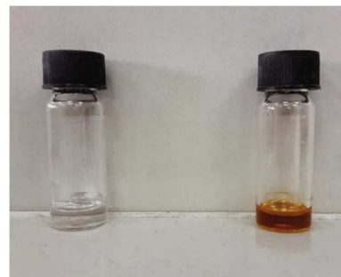
Scheme 1. NH 2 -PEG x -NH 2 / IoE mixture at early stage (left bottle) and after two hours of stirring (right bottle).
