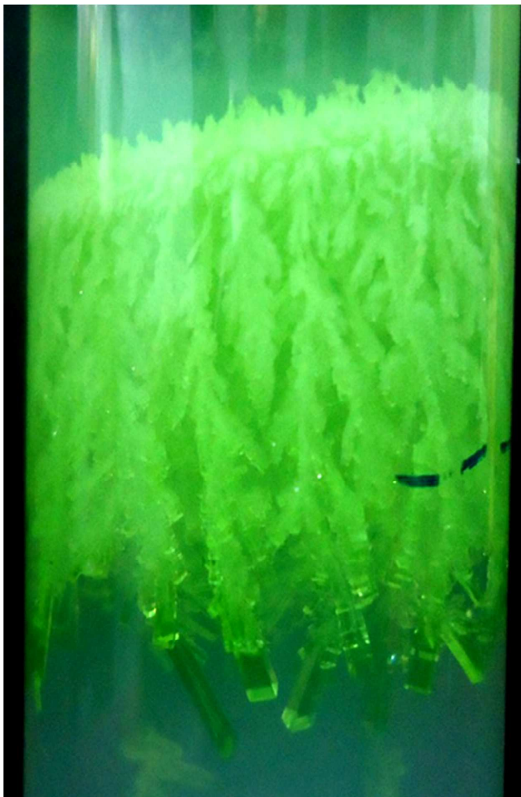
Fig.1. Single crystals of PMH developing from the tips of the dendritic formation in the gel.
