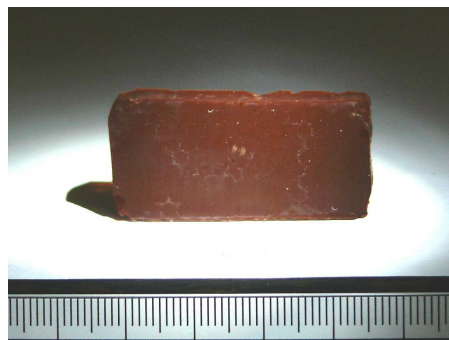
Fig. 1 Photograph of a typical aerogel sample A-(ET+H 2 O) compared to a cm scale
