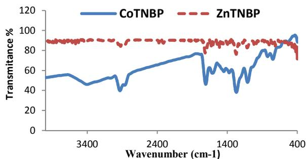
Fig 2. FT-IR spectra of metalloporphyrins
