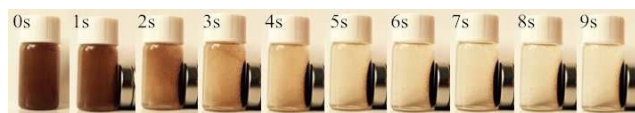
Figure 5 Separation of the IFIC MNPs by a magnet near the vessel wall in 9 seconds.
