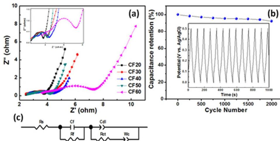
Fig. 5. (a) Nyquist plots for CF20, CF30, CF40, CF50 and CF60 electrodes within frequency range 20 kHz to 0.1 Hz (inset: magnified image at high frequency region), (b) variation of capacitance retention and cycle number (Inset: charge discharge curves), (c) The electrical equivalent circuit used for fitting impedance spectra
