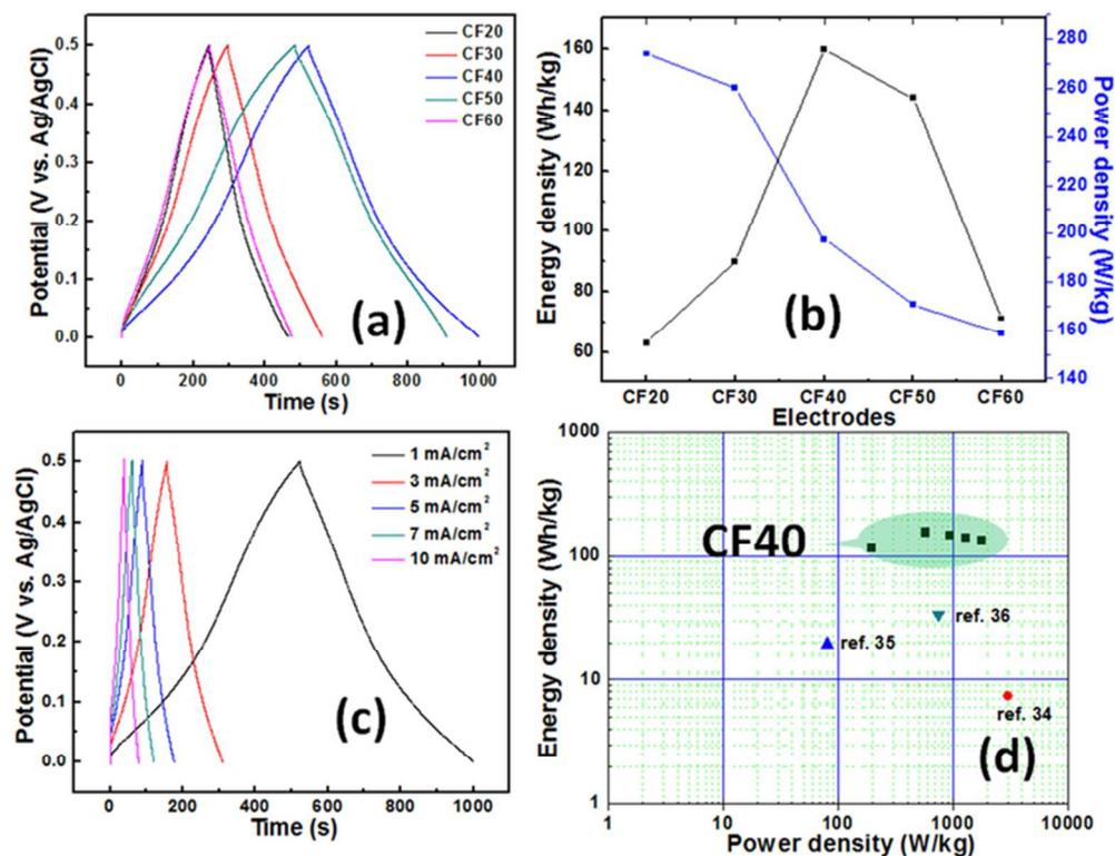
Fig. 4. (a) Charge discharge curves of CF20, CF30, CF40, CF50 and CF60 electrodes at the current density of 1 A/g; (b) variation of energy and power densities with mass loading of each electrode; (c) Charge discharge curves for CF40 electrode at the current densities of 1, 3, 5, 7 and 10 A/g; (d) Ragone plot for CF40 electrode compared with literature values.
