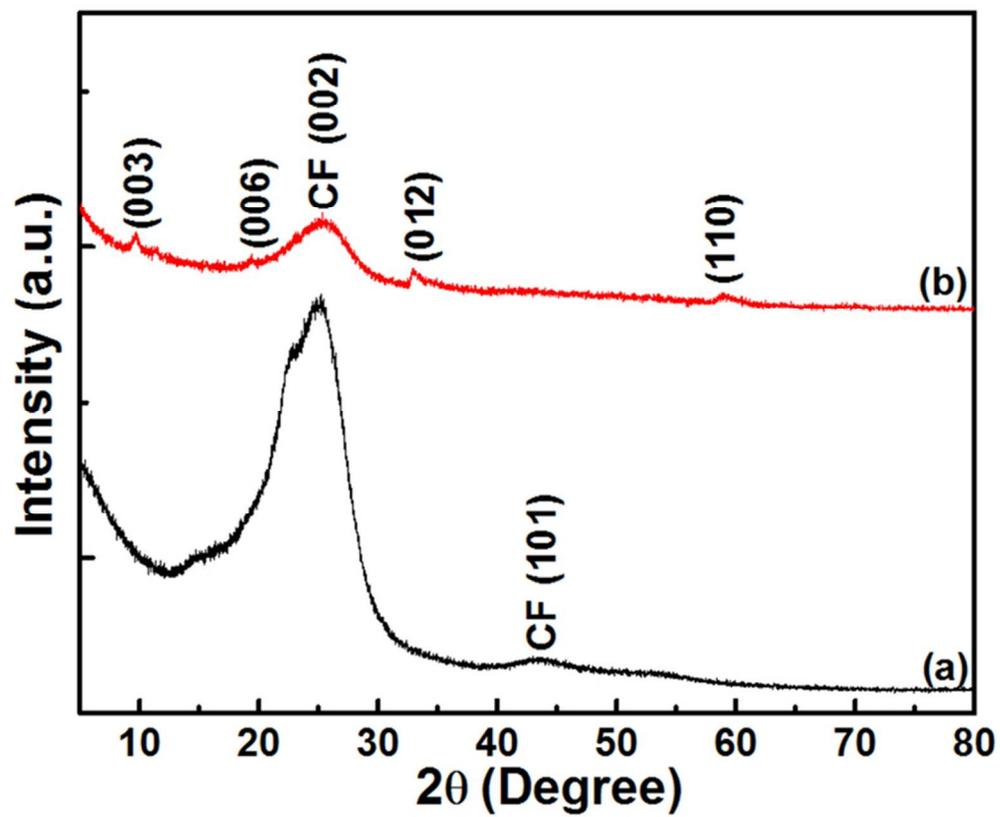
Fig. 2. XRD patterns of (a) bare CF and (b) CF40 samples.
