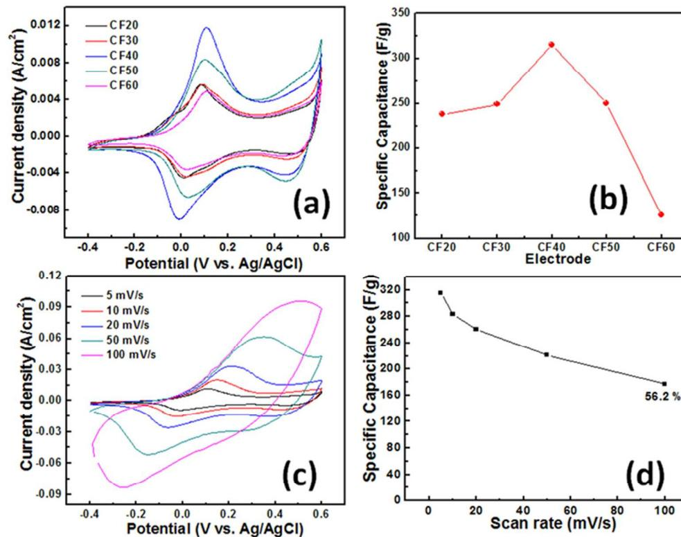
Fig. 3. (a) CV curves of CF20, CF30, CF40, CF50 and CF60 electrodes at the scan rate of 5 mV/s; (b) variation of specific capacitance with mass loading of each electrode; (c) CV curves of CF40 electrode at scan rates of 5, 10, 20, 50 and 100 mV/s; (d) specific capacitances of CF40 electrode at scan rates of 5, 10, 20, 50 and 100 mV/s.
