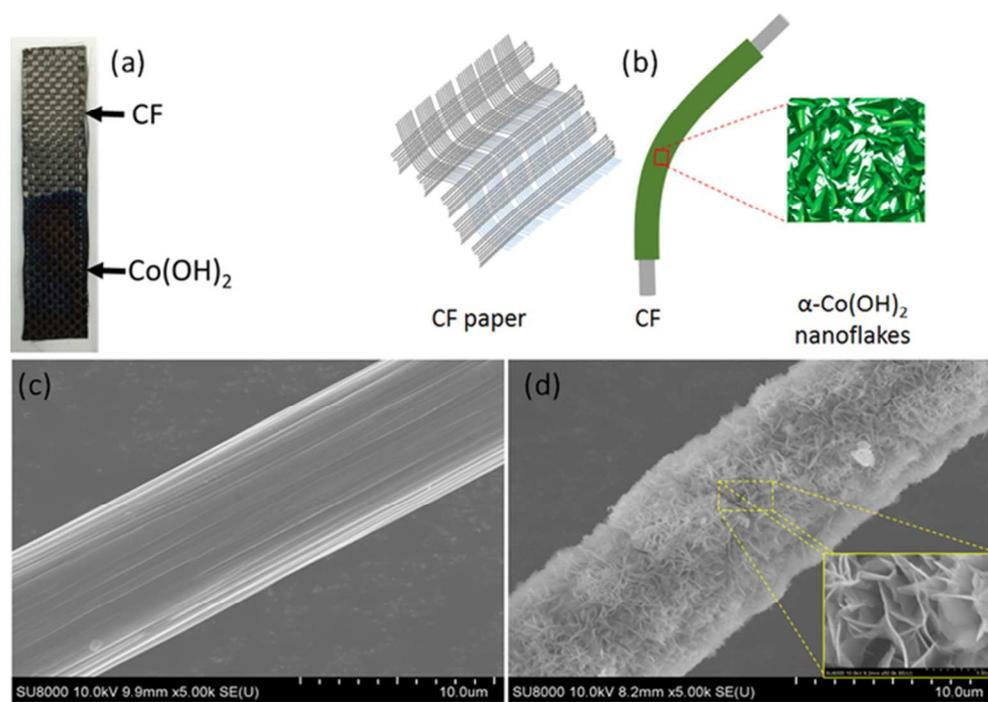
Fig. 1. (a) Photograph of CF paper coated with cobalt hydroxide nanoflakes. (b) Schematic diagram illustrating the loading procedure of cobalt hydroxide on CF. (c) SEM image of bare CF. (d) SEM image of cobalt hydroxide nanoflakes coated on CF. Inset: magnified SEM image of the nanoflakes. 57x40mm (300 x 300 DPI)
