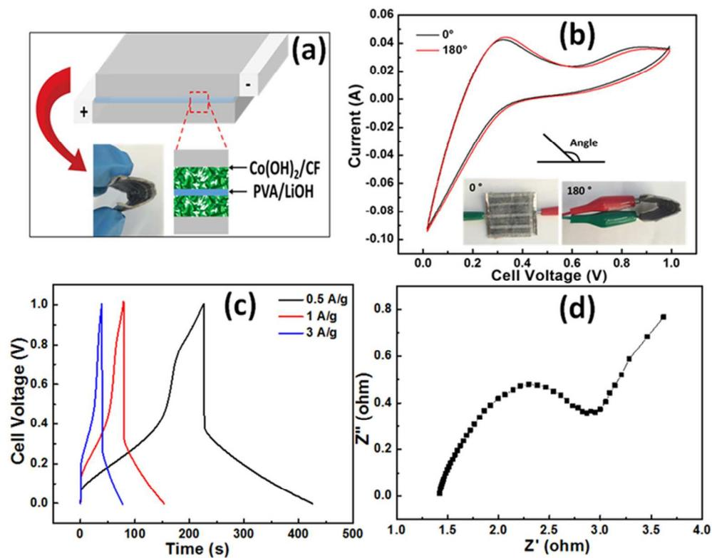
Fig. 6 (a) Schematic of flexible supercapacitor fabrication, (b) CV curves at bending conditions of  $0^\circ$  and  $180^\circ$  at scan rate of 20 mV/s, (c) Charge-discharge curves at current densities of 0.5, 1 and 3 A/g, (d) Nyquist plot for the supercapacitor within frequency range 105 Hz to 0.1 Hz.
