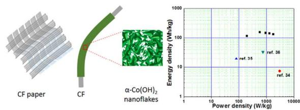
Present work states about successful loading of  $\text{Co(OH)}_2$  on carbon fiber paper as an electrode for high performance flexible supercapacitor.
