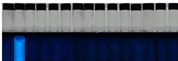
Fig. 7. Colour change of 3 upon interaction with tested cations (top: under natural light; bottom: under UV light). From left to right: Blank, \text{Cr}^{3+} , \text{Ag}^+ , \text{Al}^{3+} , \text{Ba}^{2+} , \text{Cd}^{2+} , \text{Cu}^{2+} , \text{Fe}^{3+} , \text{Hg}^{2+} , \text{K}^+ , \text{Mn}^{2+} , \text{Na}^+ , \text{Ni}^{2+} , \text{Pb}^{2+} , \text{Zn}^{2+} .
