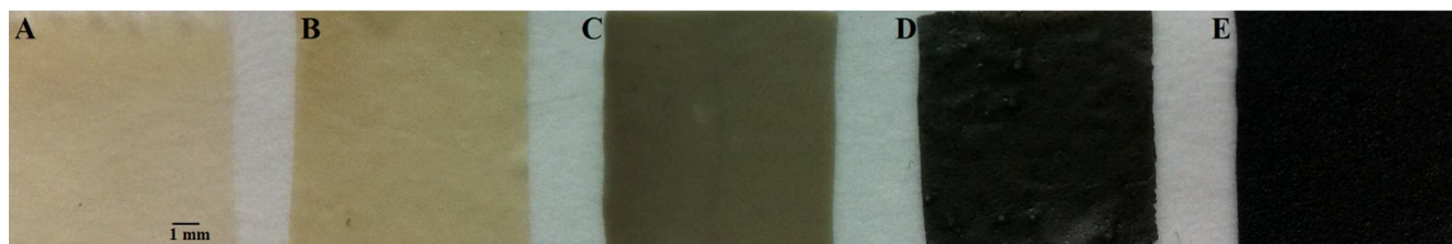
Fig. 3 The photographs of the membranes with different amounts of MWCNTs. A: CP-MIM3 (0%); B: CP/DA-MIM2 (0%); C: CP/CNT/DA-MIM1 (0.5%); D: CP/CNT/DA-MIM2 (1%); E: CP/CNT/DA-MIM3 (1.5%).
