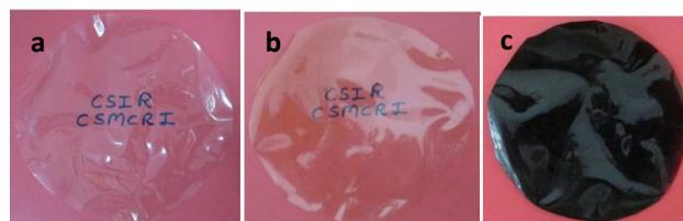
Fig. 5 Images of the hybrid sample cured at 60 °C (a), the sample M3-T1 cured at 150 °C after prior heating at 60 °C (b) and the sample M3-T2 cured directly at 150 °C (c).
