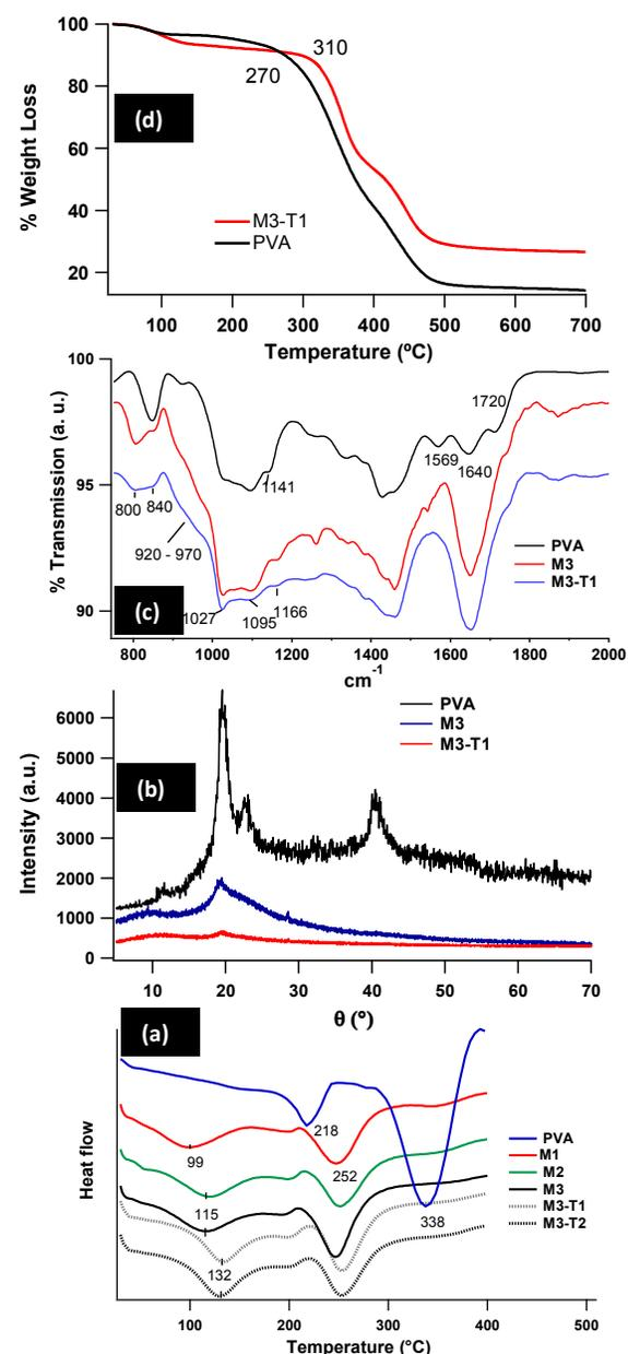
Fig. 7 DSC plots (a), XRD patterns (b), FT-IR spectra (c) and TGA plots (d) showing differences between the hybrid sample and neat poly(vinyl alcohol) (PVA) sample
