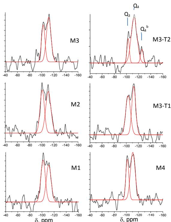
Fig 2  $^{29}\text{Si}$  NMR spectra of the silica-poly(vinyl alcohol) hybrid membranes films
