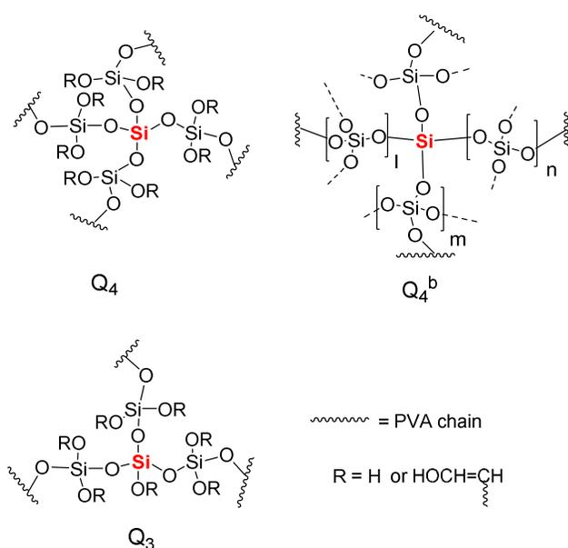
Fig. 3 Probable connectivity of  $\text{SiO}_4$  tetrahedral units with PVA chains
