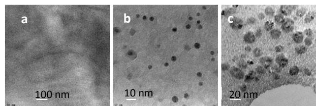
Fig. 4 TEM images of the hybrid sample cured at 60 °C (a), the sample M3-T1 cured at 150 °C after prior heating at 60 °C (b) and the sample M3-T2 cured directly at 150 °C (c).
