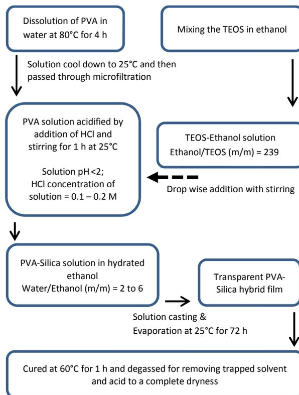
Fig 1 Membrane preparation scheme
