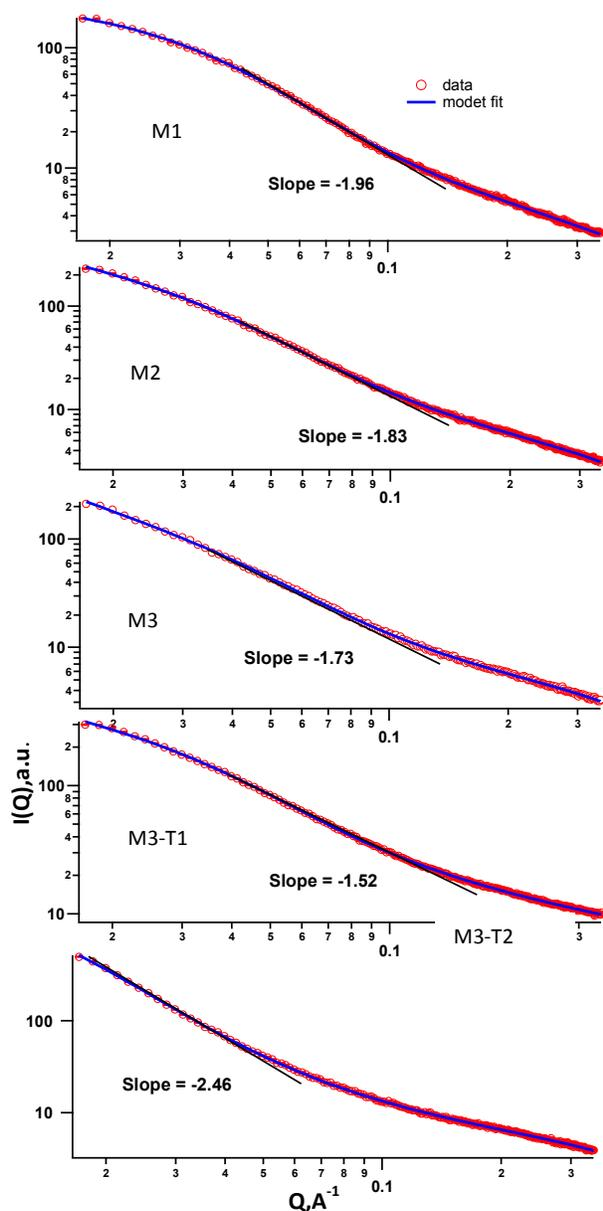
Fig. 6 SAXS profiles of the hybrid samples. Solid lines indicate DAB model fits
