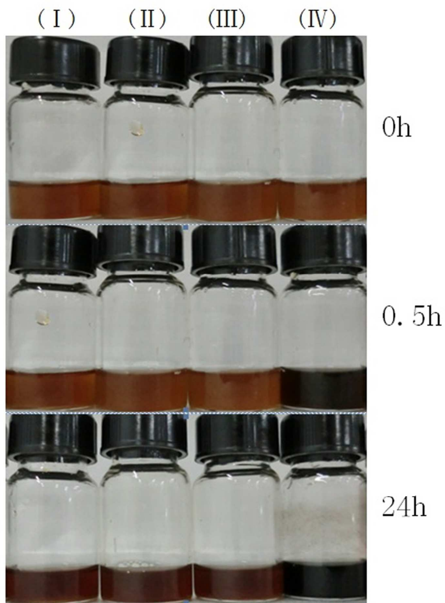
Time-course digital photographs of GO reduction with different reaction conditions: (I) blank control, (II) redox mediator (VK3), (III) B. subtilis 168, (IV) B. subtilis 168 with redox mediator (VK3) 111x148mm (300 x 300 DPI)
