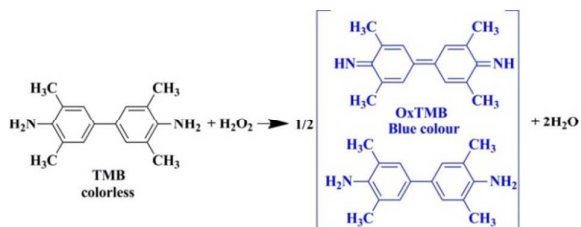
Scheme 1 The oxidation reaction of TMB by compound 1 or 2 in the presence of \text{H}_2\text{O}_2 .
