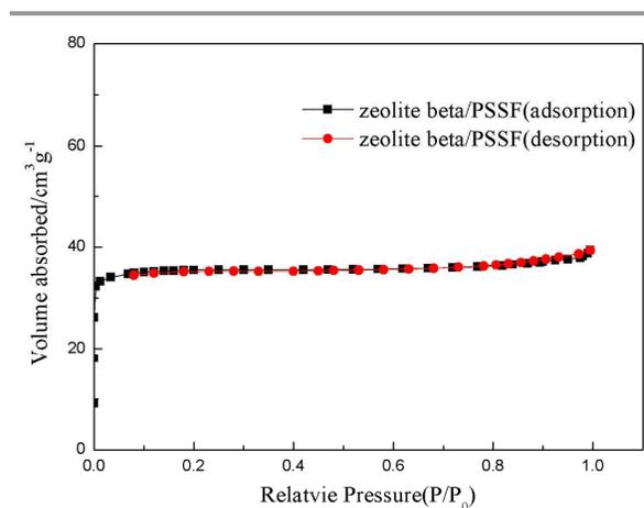
Fig. 4.  $\text{N}_2$  adsorption/desorption of the zeolite beta coating/PSSF composite at 77K.
