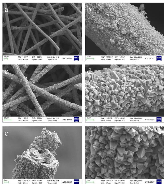
Fig. 2. SEM images of paper-like stainless steel fibers (a); the zeolite beta seeds layer (b); morphology of zeolite beta coating/PSSF composite (c); morphology of zeolite beta coating on stainless steel fibers (d), (e) and (f).
