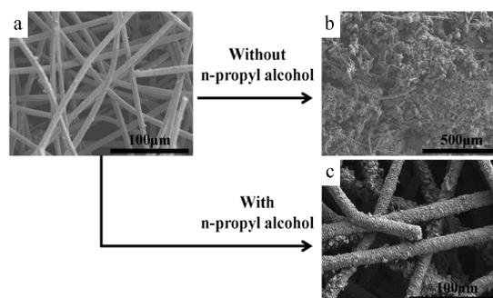
Fig. 1. SEM images of paper-like stainless steel fibers support (a); secondary synthesis of zeolite beta coating on stainless steel fibers without (b) and with (c) n-propyl alcohol in fluoride media.
