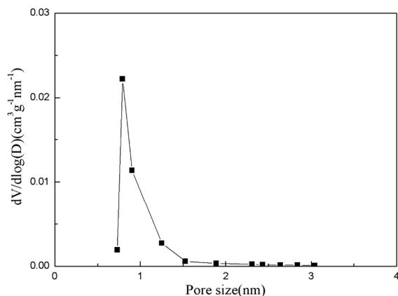
Fig. 5. Pore size distribution of the zeolite beta coating/PSSF composite.
