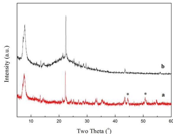
Fig. 3. X-ray diffraction patterns of different samples: (a) zeolite beta coating/PSSF composite; (b) samples deposited on the bottom of the autoclave.
