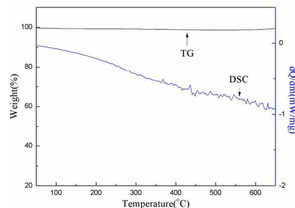
Fig. 6. TG-DSC curves of the zeolite beta coating/PSSF composite.
