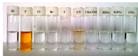
Figure 5 Change in colour of H1 (20 μM) in dry DMSO after the addition of 10 equivalents of tetrabutylammonium salt of anions.
