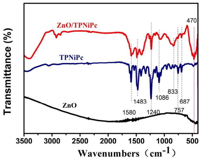
Figure 2. FTIR spectra of ZnO–NRs/TPNiPc hierarchical hetero-nanostructures, TPNiPc and ZnO–NRs.
