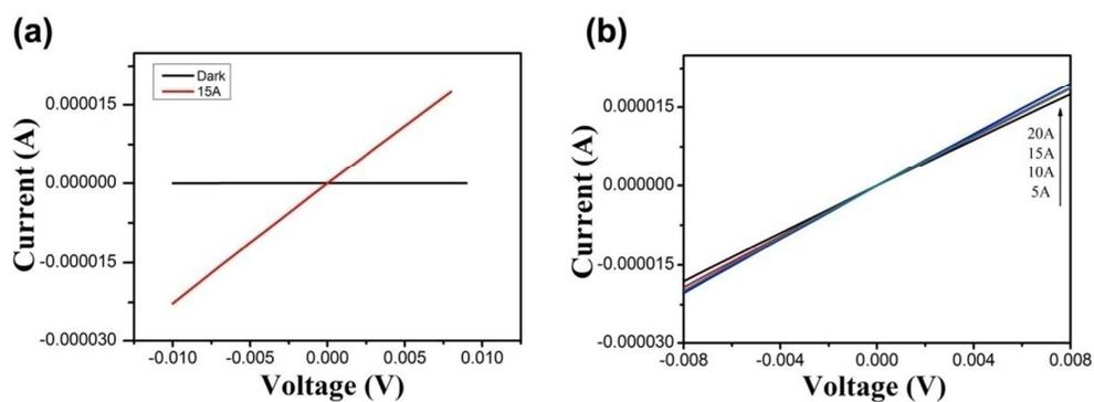
Figure 8. (a) *I-V* curves of ZnO-NRs/TPNiPc hierarchical hetero-nanostructure arrays measured in dark and under illumination by using a 300 W Xe lamp (15A), respectively; (b) Photocurrents of the ZnO-NRs/TPNiPc hierarchical hetero-nanostructure arrays under the visible light of different power.
