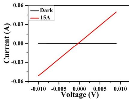
Figure 9.  $I$ - $V$  curves of ZnO-NRs/TPNiPc hierarchical hetero-nanostructure arrays assisted with  $\text{H}_2\text{O}_2$  measured in dark and under illumination by using a 300 W Xe lamp (15A), respectively.
