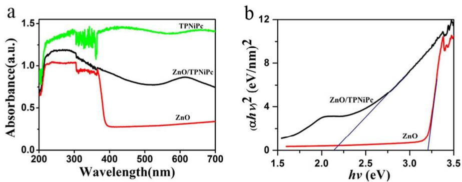
Figure 7. (a) UV-vis diffuse reflectance spectra of the as-prepared ZnO-NRs/TPNiPc hierarchical hetero-nanostructures, TPNiPc and ZnO-NRs at room temperature. (b) Plots of the  $(\alpha h\nu)^2$  vs. vs. photon energy ( $h\nu$ ) for the as-obtained samples.
