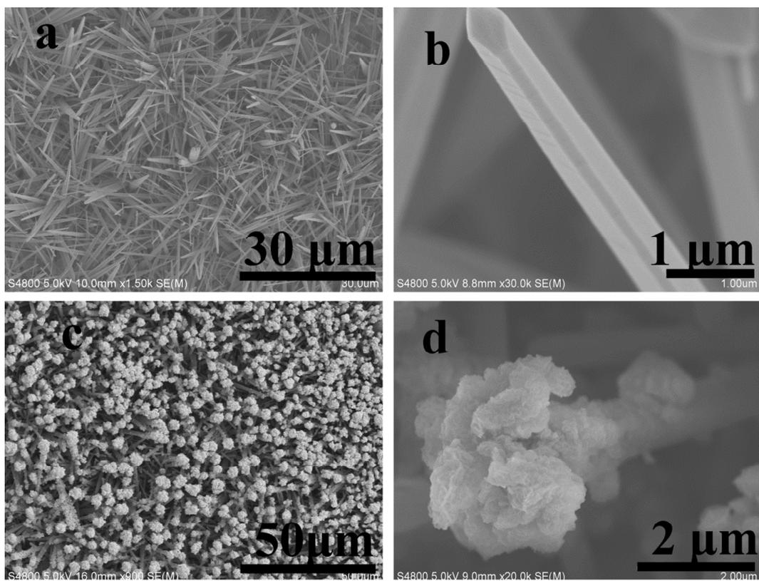
Figure 3. (a, b) FESEM images of ZnO-NRs; (c, d) FESEM images of the ZnO-NRs/TPNiPc hierarchical hetero-nanostructures.
