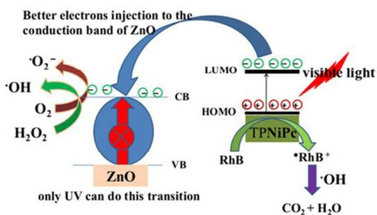
**Scheme 2.** Illustrative diagram for the photocatalytic mechanism of ZnO–NRs/TPNiPc hierarchical hetero-nanostructure assisted with  $\text{H}_2\text{O}_2$ , VB = valence band, CB = conduction band, HOMO = highest occupied molecular orbital and LUMO = lowest occupied molecular orbital.
