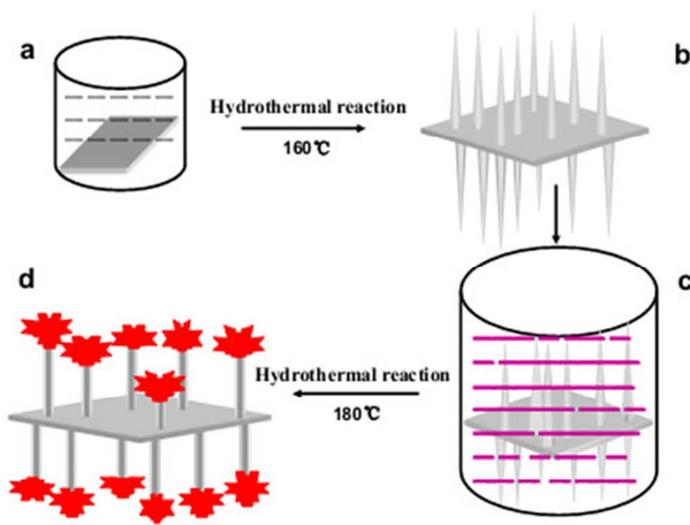
**Scheme 1.** Schematic illustration of the fabrication of the ZnO-NRs/TPNiPc hierarchical heteronanostructures: (a) zinc foil was inserted into the first solution; (b) needle-like ZnO-NRs grew on both sides of zinc foil; (c) ZnO-NRs covered on zinc foil was inserted into the second solution; (d) TPNiPc hierarchical hetero-nanostructure assembled onto the top of needle-like ZnO-NRs.
