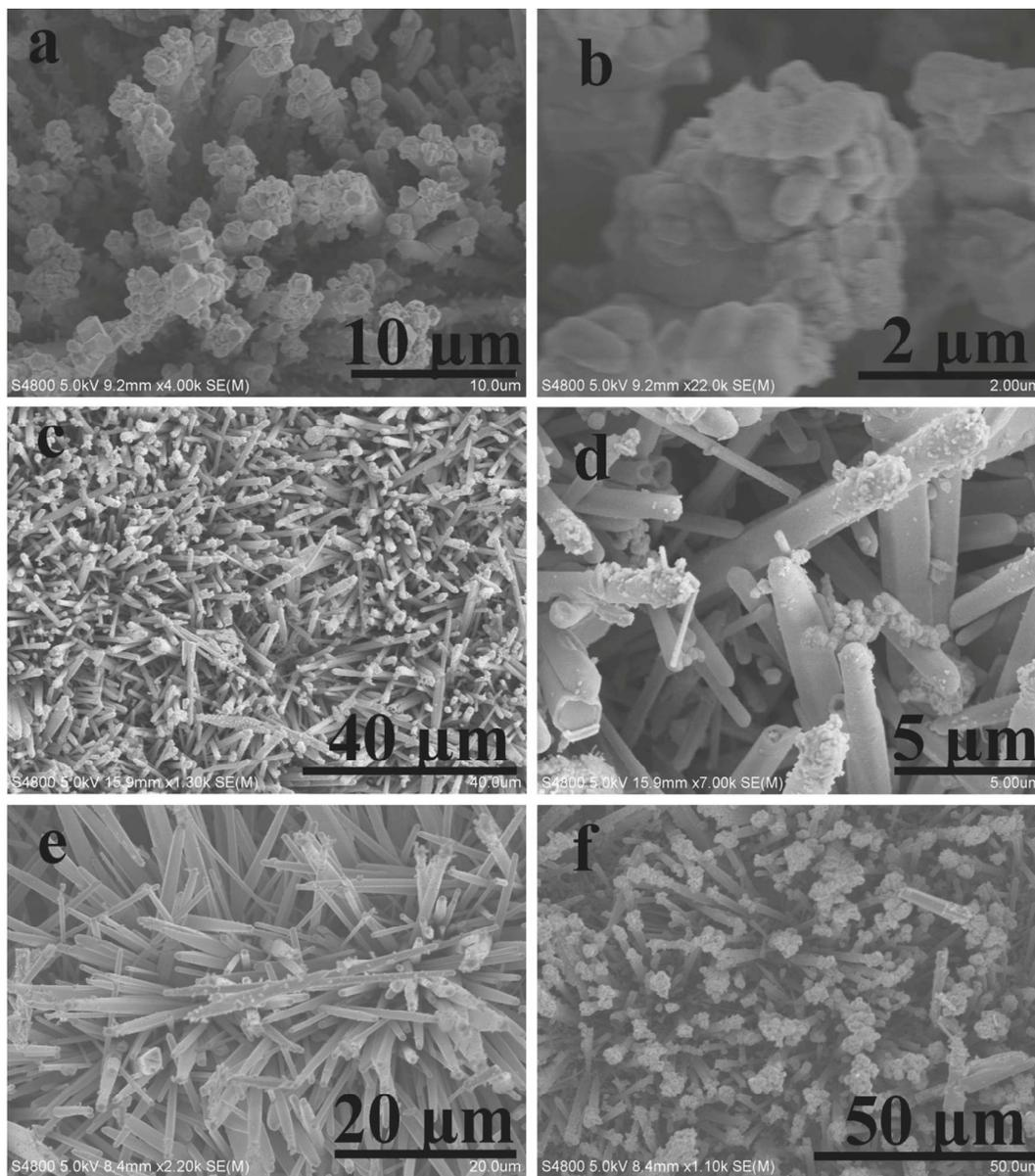
Figure 4. FESEM images of the ZnO-NRs/TPNiPc hierarchical hetero-structures attained at different reaction conditions: (a, b) at 200 °C; (c, d) the dosage of 4-Phenoxyphthalonitrile is 0.025 g; (e) the heating time is under 5 h; (f) the heating time is about 10 h.
