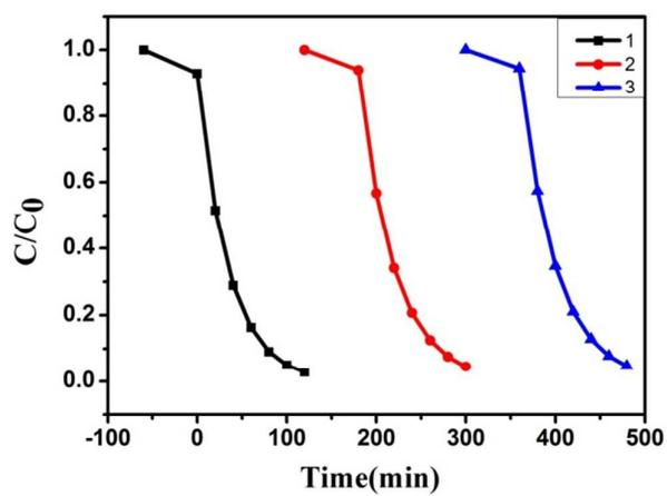
Figure 6. Cycling runs for the photodegradation of RhB by the ZnO-NRs/TPNiPc hierarchical hetero-nanostructure arrays assisted with  $H_2O_2$  under visible light irradiation.
