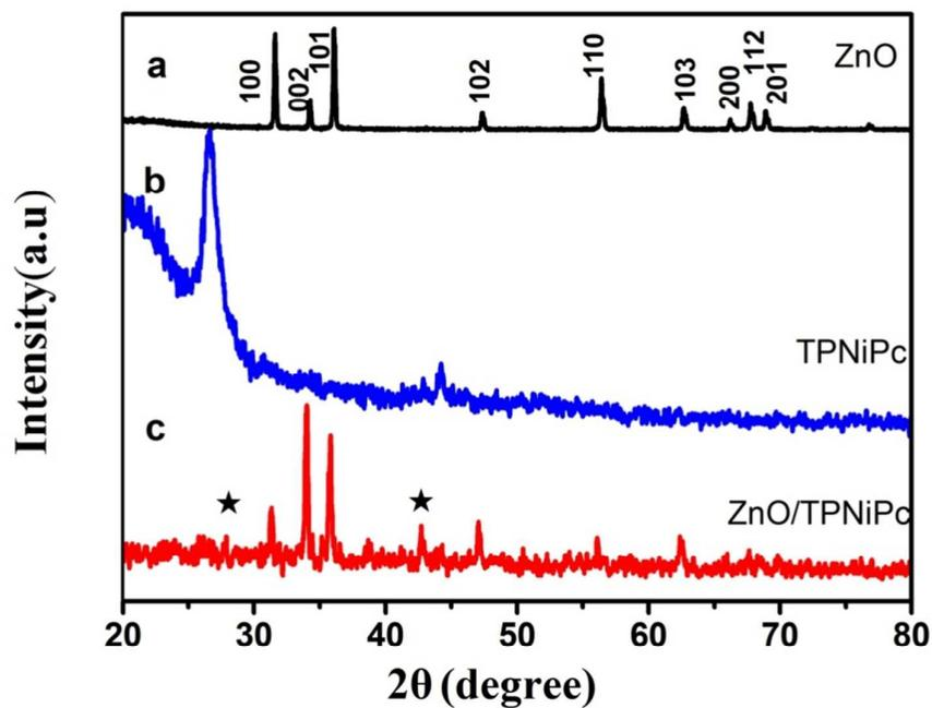
Figure 1. XRD patterns of ZnO–NRs/TPNiPc hierarchical hetero-nanostructures, TPNiPc and ZnO–NRs.
