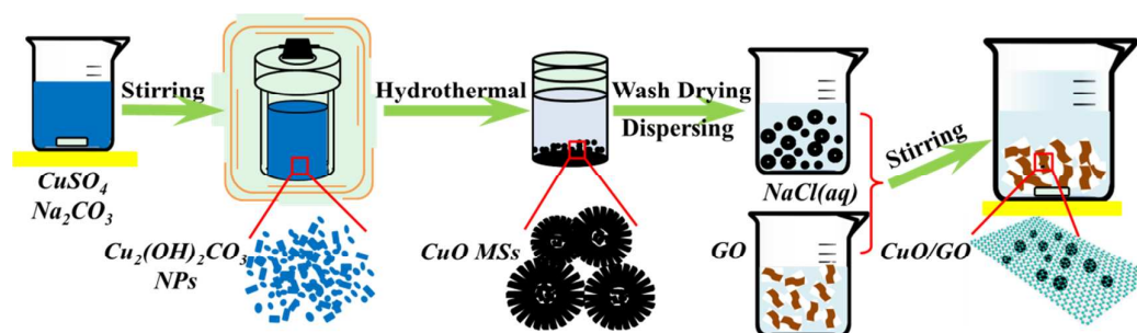
Fig. 6 Schematic illustration of the synthesis process for CuO MSs and CuO/GO hybrid.
