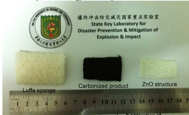
**Fig. 1** Digital photo of luffa sponge, carbonized product and as-prepared ZnO structure.
