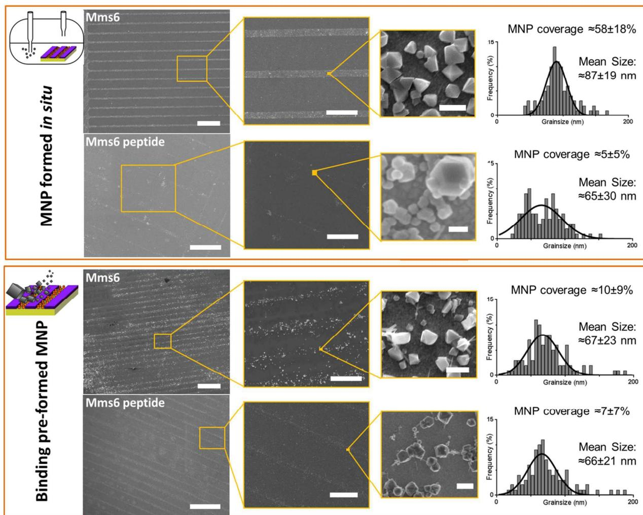
Fig. 5: SEM analysis of the different surfaces at increasing magnification. Scale bars are 100 μm (left), 20 μm (centre), and 100 nm (right). MNP sizing histograms are shown with Gaussian fitting (GraphPad Prism). MNP coverage from 5 areas of biomolecule patterned regions is shown for each sample with standard deviation.
