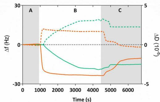
Fig. 2. Frequency ( $\Delta f$ , solid lines) and dissipation ( $\Delta D$ , dotted lines) changes of the 7th overtone recorded with QCM-D during adsorption of cys-Mms6 (green) or cys-pep (orange) onto clean gold coated quartz crystals. Grey regions show when a Milli-Q water buffer was applied (A and C), and white regions (B) show when a PBS buffer containing cys-Mms6 or cys-pep at a concentration of  $10 \mu\text{g mL}^{-1}$  was applied (flow rate  $50 \mu\text{L min}^{-1}$ ).
