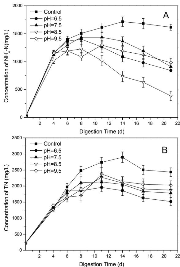
Fig. 4. Variations of (A)  $\text{NH}_4^+$  and (B) TN in the supernatant of simulated one-stage ATAD systems.
