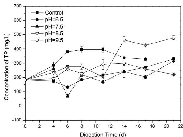
Fig. 5. Changes of TP in the supernatant of simulated one-stage ATAD systems.
