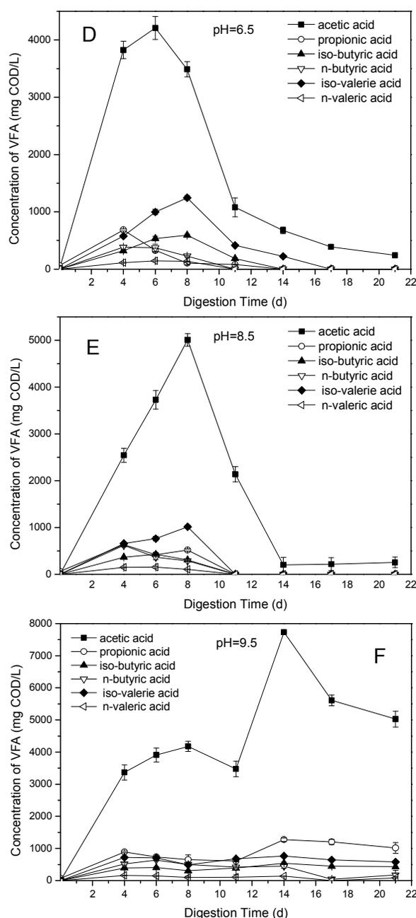
Fig. 3. Changes of (A) SCOD; (B) TVFA {total VFAs}; (C) individual VFA of the control; (D) individual VFA of pH 6.5; (E) individual VFA of pH 8.5; (F) individual VFA of pH 9.5 in the supernatant of simulated one-stage ATAD systems.
