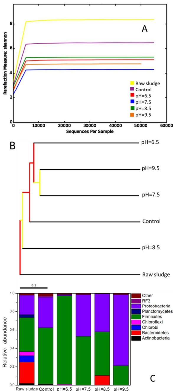
Fig. 6. Results of Illumina high throughput sequencing: (A) Shannon rarefaction curves; (B) clustering tree; (C) taxonomic compositions of bacterial communities at phylum level in the simulated one-stage ATAD systems. Relative abundance was defined as the number of sequences affiliated with that OTU divided by the total number of sequences per sample. The relative abundance of phyla less than 1.0% of total composition in the three libraries was defined as “other”.
