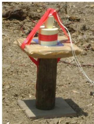
**Fig.12.** Trial set up for Shock Sensitivity Test
