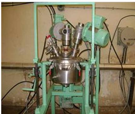
**Fig.1.** Steam Jacketed Anchor Blade Mixer
