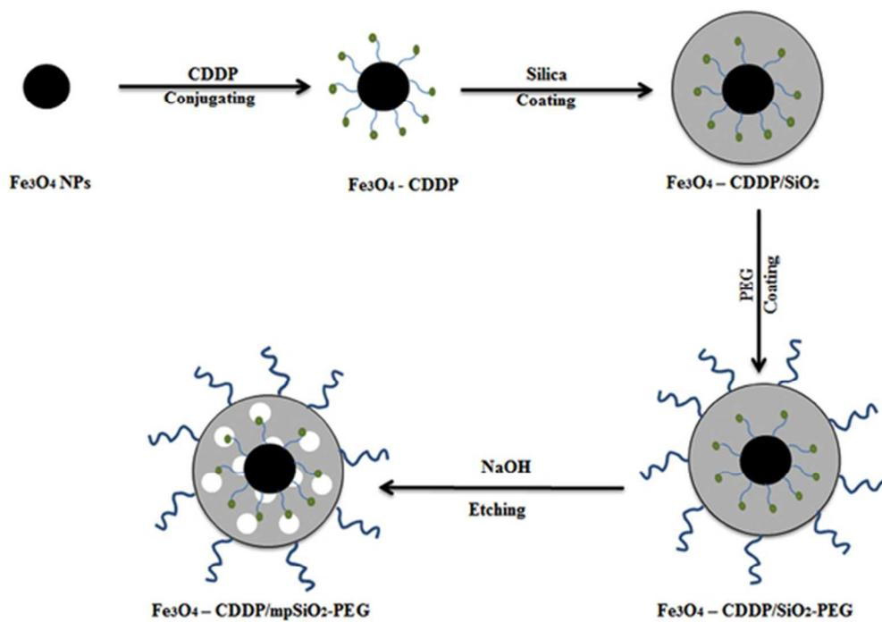
Scheme 1 Schematic representation of the synthesis of the magnetic drug delivery nanosystem composed of Fe<sub>3</sub>O<sub>4</sub>-CDDP conjugation cores and a PEG-functionalized porous silica shell.
