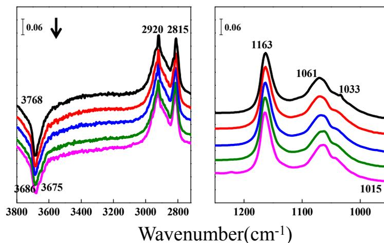
**Fig. 5** Infrared spectra of methanol desorption on zirconium sample
