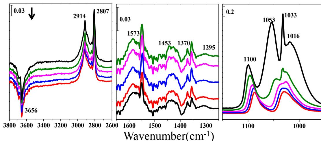
**Fig. 4** Infrared spectra of methanol desorption on ceria sample
