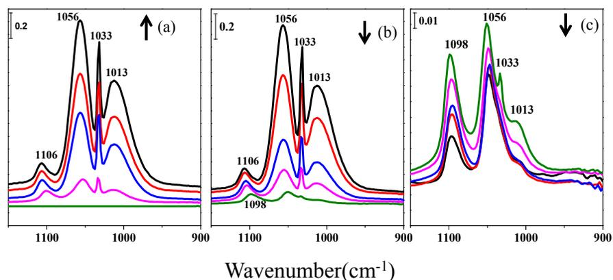
**Fig. 3** Infrared spectra of methanol adsorption and desorption on mixed sample: (a) methanol adsorption (b) methanol desorption in He stream (c) methanol desorption under evacuation
