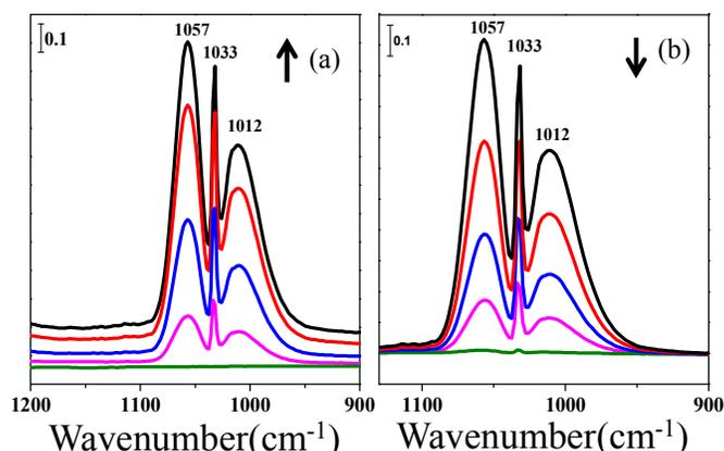
**Fig. 2** Infrared spectra of methanol adsorption and desorption on CaF<sub>2</sub>: (a) methanol adsorption (b) methanol desorption in He stream
