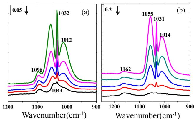
**Fig. 1** Infrared spectra of catalysts containing preadsorbed methanol exposed in He stream for 0.5 h (a) CeO<sub>2</sub> (b) ZrO<sub>2</sub>
