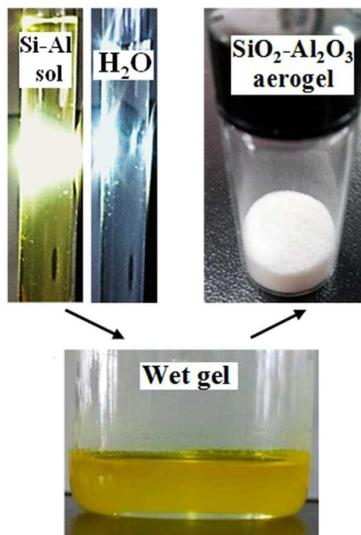
The SiO<sub>2</sub>-Al<sub>2</sub>O<sub>3</sub> aerogel has been synthesized using coal gangue as a raw material via ambient pressure drying method.
