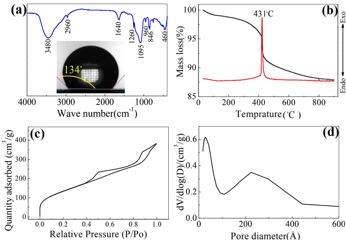
**Fig. 4.** (a) FTIR spectrum of  $\text{SiO}_2\text{-Al}_2\text{O}_3$  aerogel. Inset of Fig. 4(a) is the contact angle of  $\text{SiO}_2\text{-Al}_2\text{O}_3$  aerogel with water. (b) TG-DSC curve of  $\text{SiO}_2\text{-Al}_2\text{O}_3$  aerogel in air. (c)  $\text{N}_2$  adsorption–desorption isotherms of  $\text{SiO}_2\text{-Al}_2\text{O}_3$  aerogel. (d) Pore size distribution of  $\text{SiO}_2\text{-Al}_2\text{O}_3$  aerogel.
