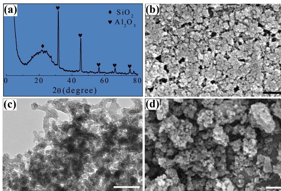
**Fig. 3.** (a) XRD pattern of the SiO<sub>2</sub>-Al<sub>2</sub>O<sub>3</sub> aerogel, (b) SEM image of the SiO<sub>2</sub>-Al<sub>2</sub>O<sub>3</sub> aerogel, and (c) TEM image of the SiO<sub>2</sub>-Al<sub>2</sub>O<sub>3</sub> aerogel. (d) SEM image SiO<sub>2</sub>-Al<sub>2</sub>O<sub>3</sub> aerogel prepared using supercritical drying method.<sup>35</sup> All of scale bars are 1μm. Reproduced with permission from ref. 35. Copyright 2005 Elsevier Inc..
