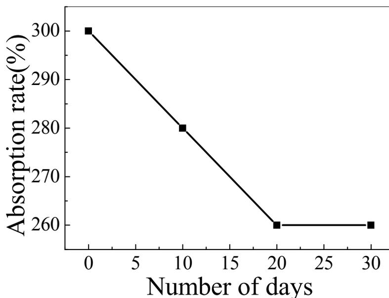
**Fig. 5.** Absorption rate tendency of  $\text{SiO}_2\text{-Al}_2\text{O}_3$  aerogel to organic solvent with time.
