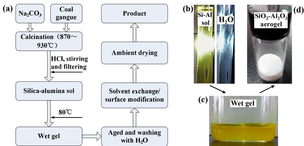
**Fig. 1.** (a) Schematic diagram of preparation of  $\text{SiO}_2\text{-Al}_2\text{O}_3$  aerogel using coal gangue as the raw materials, (b) pictures of Tyndall phenomenon of silica-alumina (Si-Al) sol by comparing with water, (c) wet gel, and (d)  $\text{SiO}_2\text{-Al}_2\text{O}_3$  aerogel.
