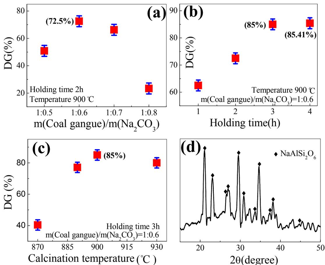
**Fig. 2.** Effects of different factors on DG: (a)  $m(\text{Coal gangue})/m(\text{Na}_2\text{CO}_3)$ , (b) holding time, and (c) calcination temperature. (d) XRD pattern of insoluble substances from reaction of coal gangue and HCl solution.
