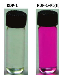
Fig. 1 Photograph showing colorimetric change during addition of \text{Pb}^{2+} to the probe RDP-1.
