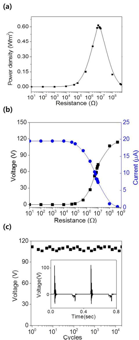
Figure 3. Electric output of a patterned triboelectric generator obtained using sandpaper (a) power density obtained for difference resistances (b) connected to the loads with different resistances, the current density and the voltage on the loads, (c) the output stability of the TEG.
