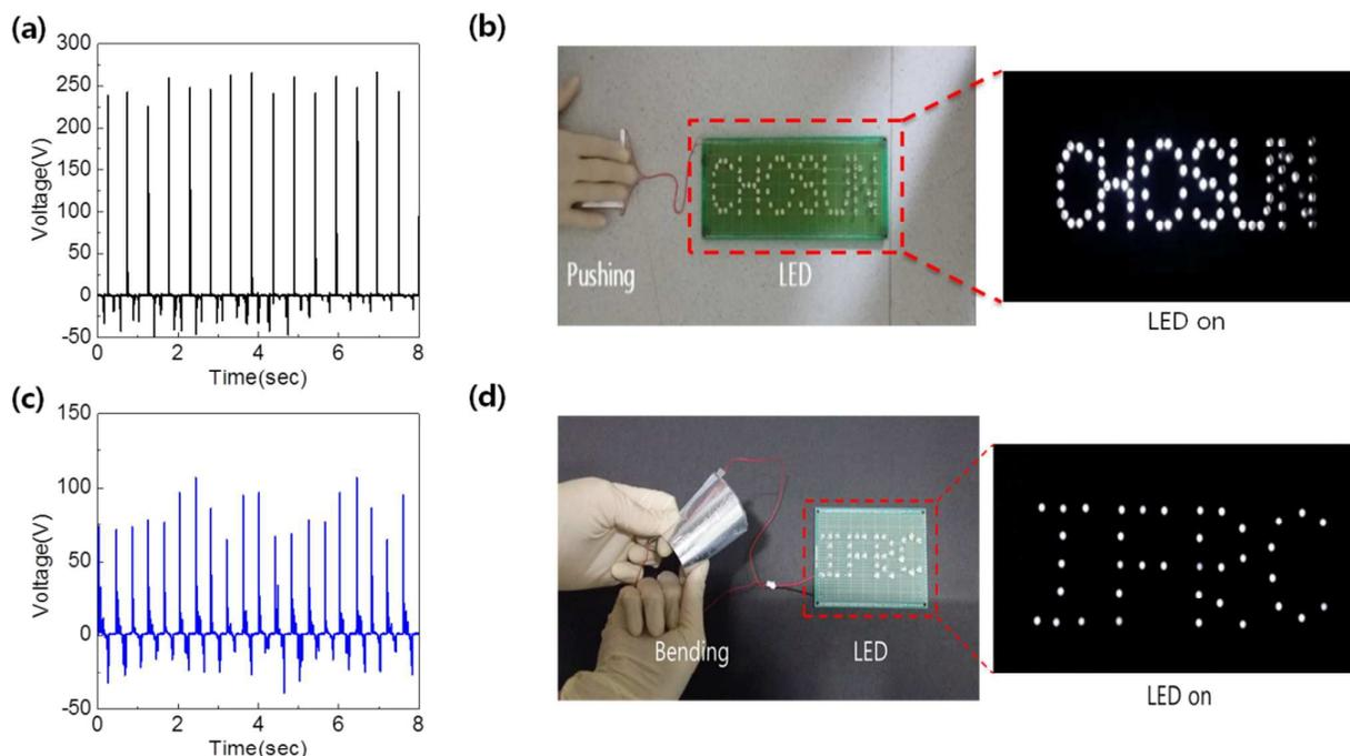
Figure 4. Performance of TEG (a) output voltage of TEG obtained by hand pushing, (b) photograph of 79 LED lamps lit using the pushing test by hand with no external circuit components, (c) output voltage of TEG obtained by hand bending, and (d) photograph of 37 LED lamps lit using the bending test by hand with no external circuit components
