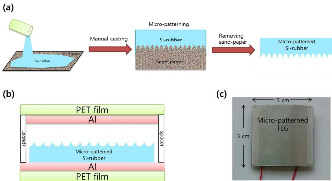
Figure 1. (a) schematic illustration of the structure and manufacture process of micropatterning PDMS (b) structure of flexible sand-patterned triboelectric generator (c) photograph of the micropatterned TEG.
