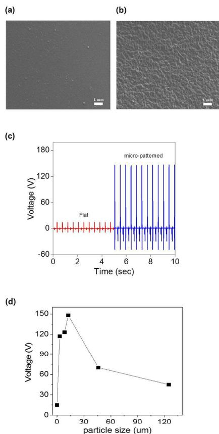
Figure 2. SEM image of (a) flat PDMS surface and (b) micropatterned PDMS surface. (c) output voltage of flat PDMS TEG and micropatterned PDMS TEG, (d) electrical performance of TEG output voltage for various particle sizes (roughness).
