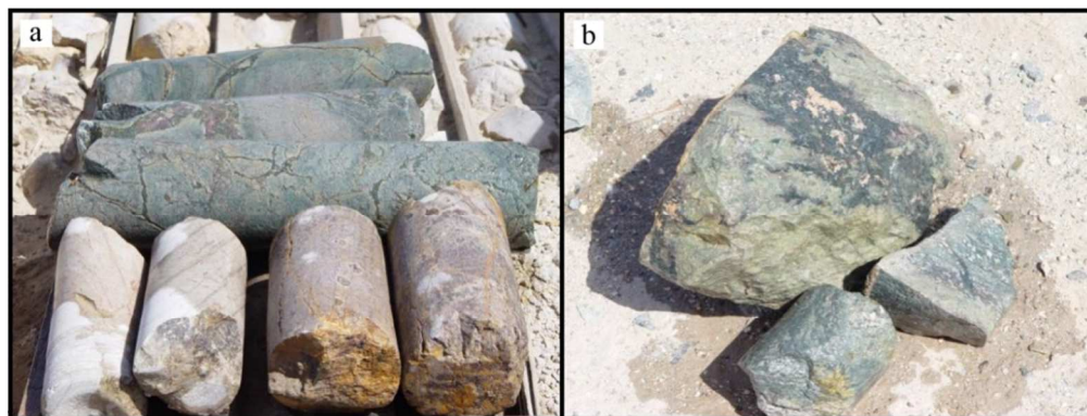
Fig. 7. The Choghartiron waste rocks. A Quartz-Albitophire and altered rhyolite in bright color and metasomatic in green color. b metasomatic rocks.
