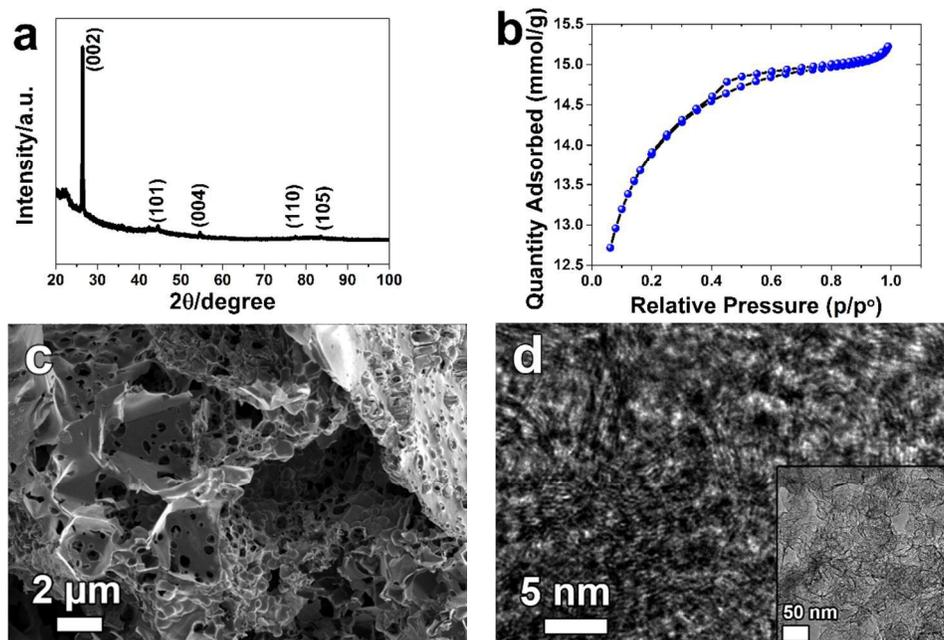
Figure 1 (a) the X-ray diffraction, (b)  $\text{N}_2$  adsorption-desorption isotherm, (c) SEM image, and (d) TEM image of AC
