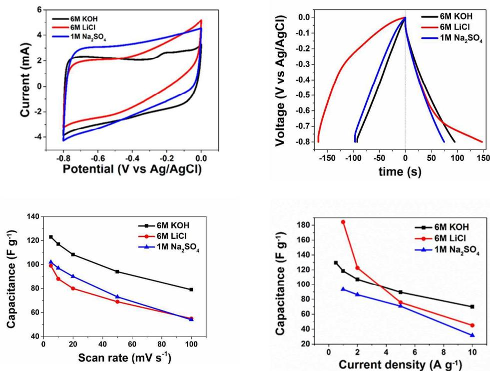
Figure 2 (a) CV curves at scan rates of  $5 \text{ mV s}^{-1}$ , (b) The galvanostatic charge/discharge curves at  $1 \text{ A g}^{-1}$ , (c) the specific capacitance as function of the scan rate and (d) the specific capacitance as function of the current density at  $0.8 \text{ V}$  of AC different for different electrolytes as shown in the figures.
