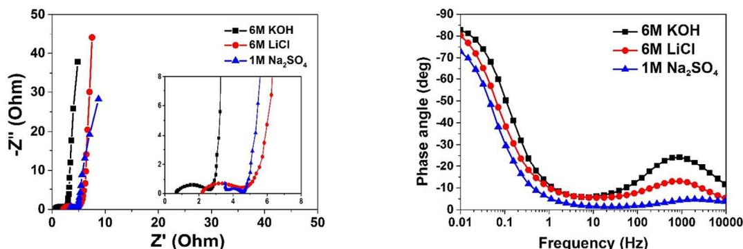
Figure 3 (a) The Nyquist plots and (b) Bode phase angle plots in different electrolytes
