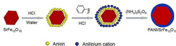
Fig.5 The simple synthesis procedure mechanism of core-shell material of PANI/SrFe 12 O 19
