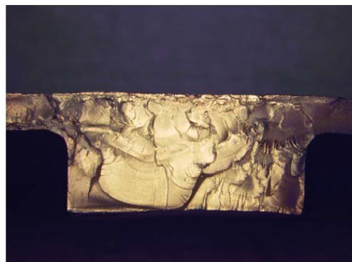
Fig. 3. Mirror housing exhibit stress cracking failure after liquid medium exposure. 22
