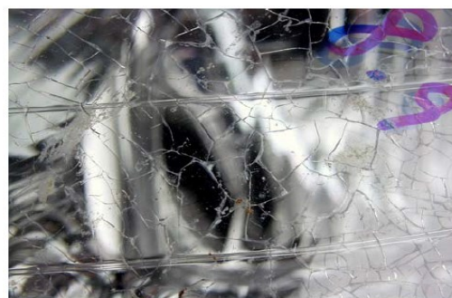
Fig. 4. Liquid medium effect on the headlight lens. 22
