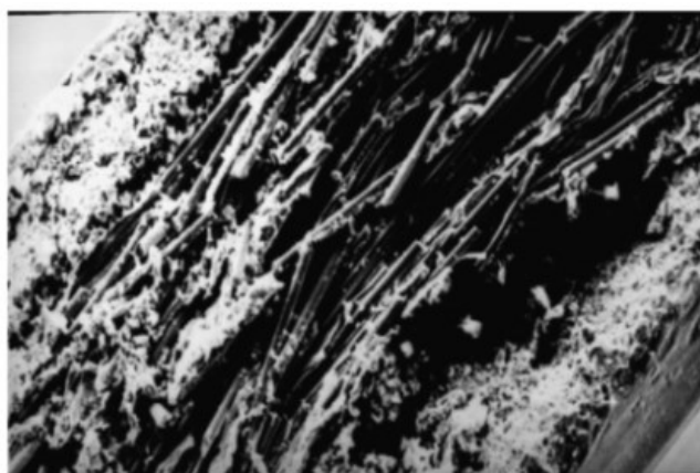
Fig. 8. Broken section of glass/polyester composite after 21-day immersion in water 14
