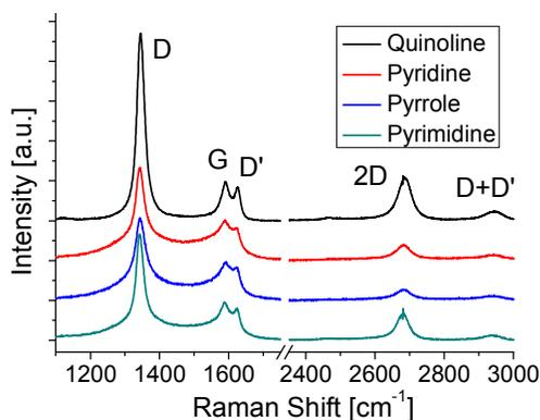
**Figure 3.** Raman spectra of N-doped graphenes synthesized at 500 °C.
