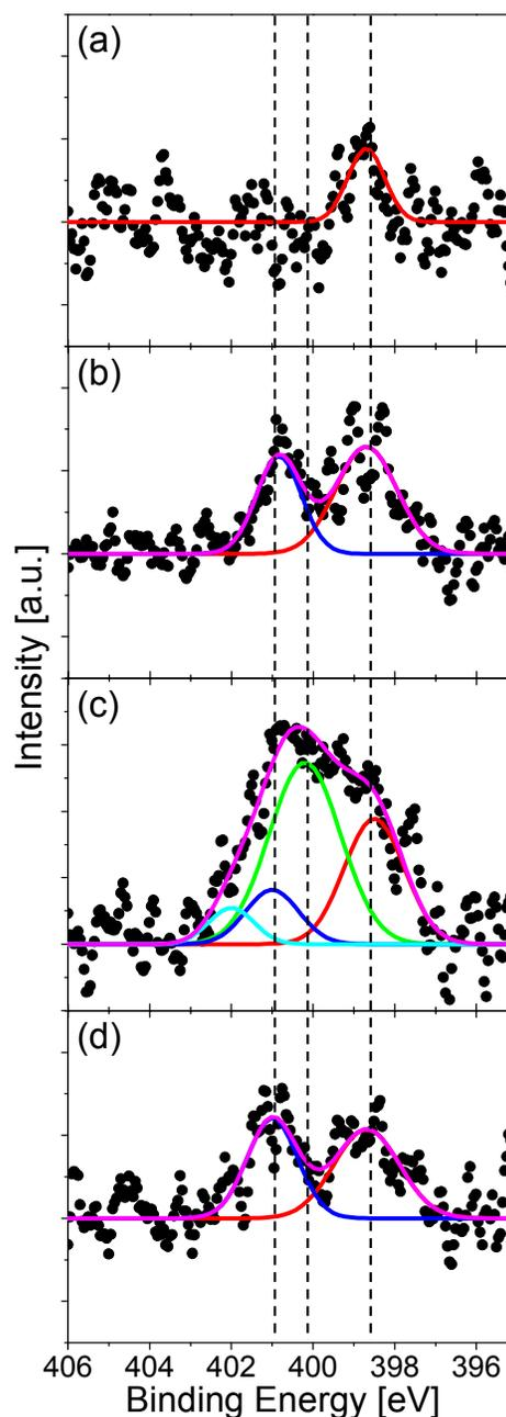
**Figure 4.** XPS N 1s spectra of N-doped graphenes synthesized at 500 °C from (a) quinoline, (b) pyridine, (c) pyrrole, and (d) pyrimidine. Each spectrum is fitted with three Gaussian functions: pyridinic- (red line), pyrrolic- (green line), and graphitic-N (blue line).
