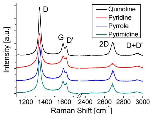
**Figure 6.** Raman spectra of the graphenes synthesized at 600 °C.
