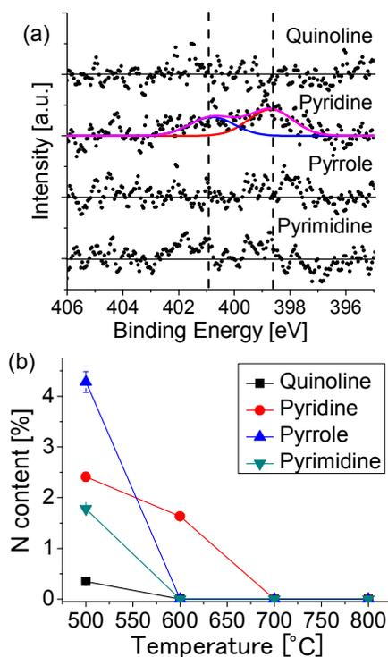
**Figure 5.** (a) XPS N 1s spectra of the graphenes synthesized at 600 °C. (b) Nitrogen content as a function of growth temperature for each of the source molecules.
