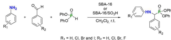
Figure 1 SBA-16 and SBA-16/SO 3 H catalyzed in a general scope of the Kabachnik-Fields reactions.
