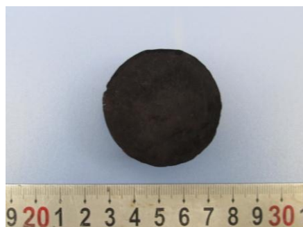
Fig. 5 Photograph of as-prepared N-doped graphene aerogels
