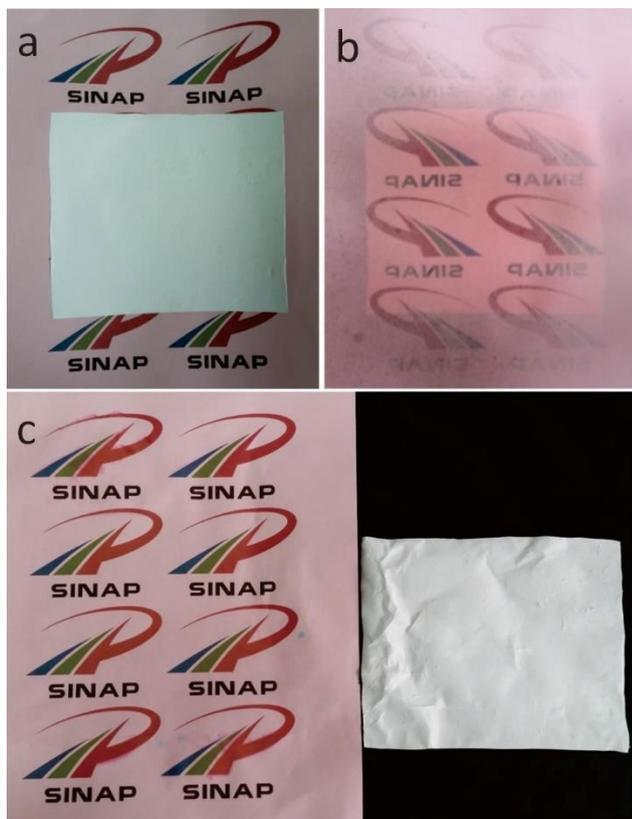
**Fig. 6** (a) A LET covered paper with a printed logos of SINAP (Shanghai Institute of Applied Physics, Chinese Academy of Sciences). (b) After spraying alcohol on the back of LET pasted paper. (c) The restored paper and LET after detaching.
