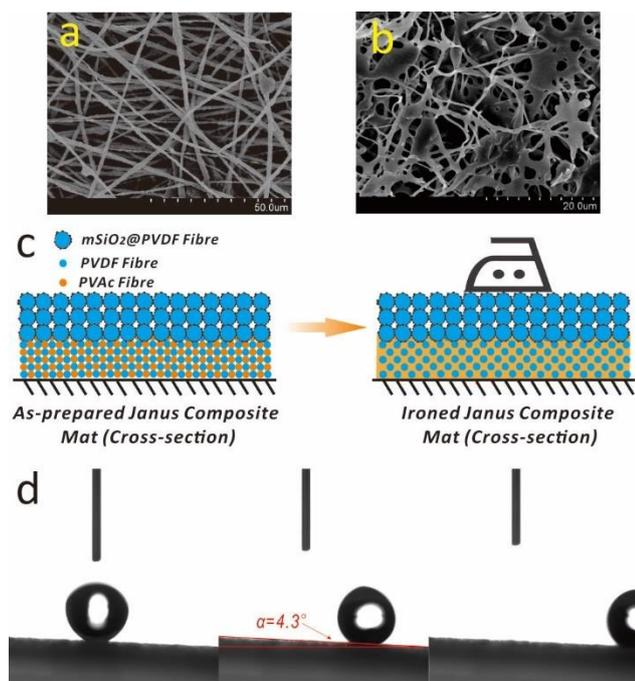
**Fig. 4** SEM images of the (a) upper and (b) bottom layer of the Janus composite mat (mass ratio: 1.0) after ironing treatment at 120 °C for 30 s. (c) The schematic program of Janus composite mats were pasted onto substrates by ironing treatment. (d) The lotus effect on glass slide pasted with Janus composite mat (mass ratio: 1.5).
