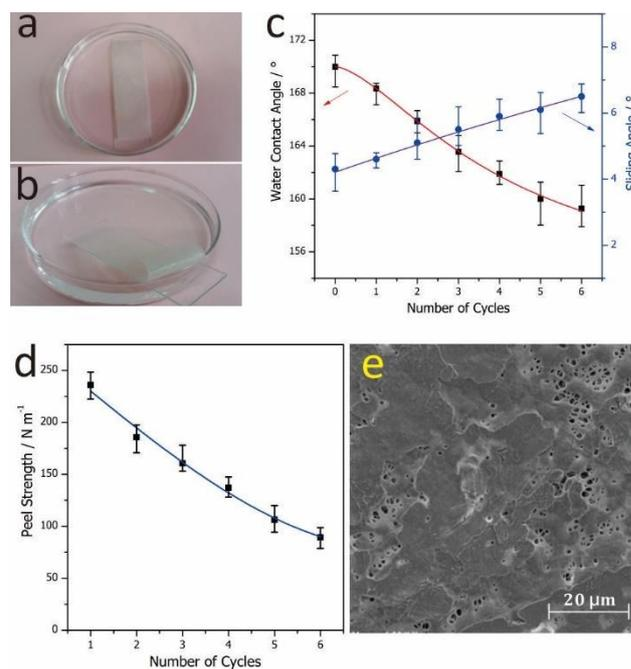
**Fig. 5** (a) Soaking of LET-pasted glass slide in ethanol for 30 s. (b) Detaching LET from glass slide after soaking in ethanol. (c) The CA and SA of LET-covered glass slides prepared with detached LET. (d) Peel strength of LET-covered glass slides prepared with detached LET. (e) SEM image of the bottom layer of the LET after 5 reusing cycles.
