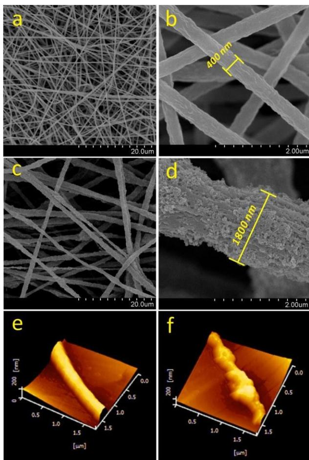
marked fluctuations on the surface, which is due to the accumulation of  $m\text{SiO}_2$  NPs undulating surface of fibres.
