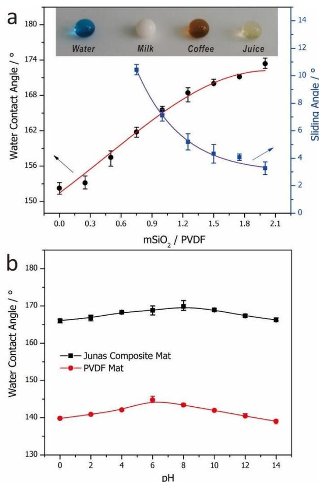
**Fig.1** (a) Water contact angles and sliding angles of electrospun Janus composite mats with different mass ratio of mSiO<sub>2</sub>/PVDF in upper layer fibres; the insert is a digital picture of different liquid droplets on the Janus composite mat (mass ratio: 1.5). (b) The stability of Janus composite mat (mass ratio: 1.5) and PVDF mat in aqueous solution with different pH.
