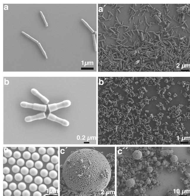
**Fig. 2.** (a and b) unassembled segmented silica rods, (a' and b') corresponding images showing failed self-assembly of rods shown in a and b, and (c) unassembled silica particles, (c') high magnification SEM image showing self-assembled silica particles, and (c'') a low magnification image showing self-assembled silica particles structures.
