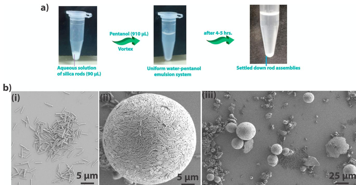
**Fig 1.** a) Schematic showing the self-assembly process, and b) (i) unassembled-smooth silica rods, (ii) self-assembled silica rod structures, and (iii) a low magnification SEM image showing intact self-assembled and broken self-assembled structures.
