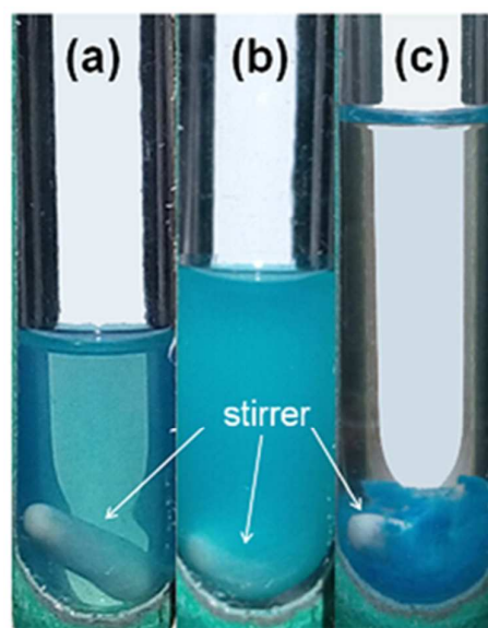
Fig. 1 Photographs of the PS-PAA@MB-ethanol system with CO 2 at (a) 0 MPa, (b) 3.20 MPa, (c) 4.75 MPa. Condition: PS-PAA concentration: 200mg/L; initial MB concentration: 3.75mg/L; temperature: 15 °C; stirring time: 1 h.
