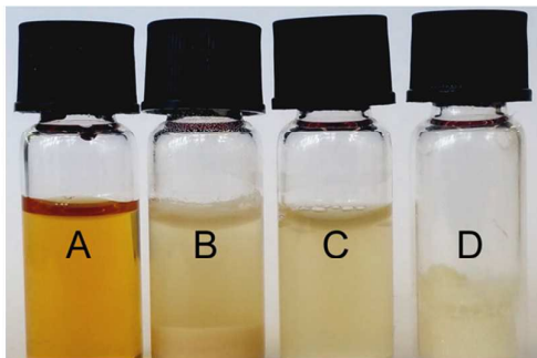
Fig. 4 Photographs at various stages of keratin extraction; namely after dissolution in eutectic (A), after dialysis showing separation of aqueous and precipitated keratin (B), extraction of the aqueous keratin (C) and subsequent freeze drying (D).
