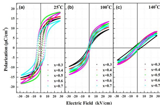
Fig.2 Ferroelectric  $P$ - $E$  loops of BZT-xBCT ceramics under  $28$   $\text{kV}/\text{cm}$  at (a)  $25$  °C, (b)  $100$  °C and (c)  $140$  °C.
