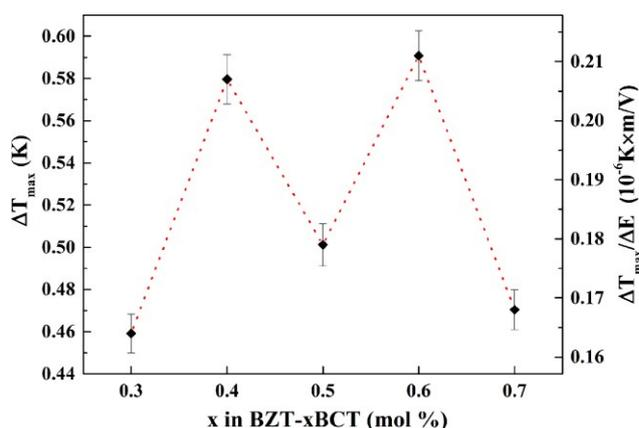
Fig.5 The maximum electrocaloric temperature change ( $\Delta T_{max}$ ) and the electrocaloric coefficient ( $\Delta T_{max}/\Delta E$ ) under 28 kV/cm ( $\Delta E = 28$  kV/cm) as a function of composition  $x$  in the BZT-xBCT system. The line is drawn as a guide to the eyes.
