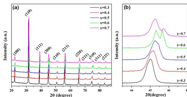
Fig. 1 (a) XRD  $\theta$ - $2\theta$  scan patterns for BZT-xBCT ceramics. (b) Evolution of pseudo-cubic  $(200)_c$  peaks as function of composition  $x$ .
