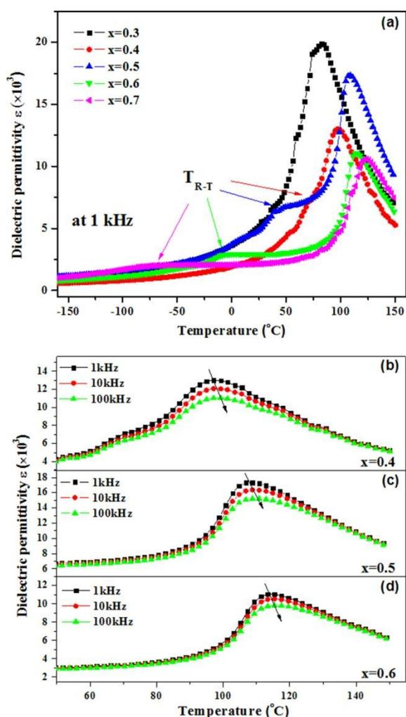
Fig.3 (a) Temperature dependence of dielectric permittivity ( $\epsilon$ ) of BZT-xBCT ceramics at 1 kHz; Dielectric permittivity as a function of temperature (50 - 150 °C) at different frequencies (1 kHz, 10 kHz and 100 kHz) for (b)  $x = 0.4$ , (c)  $x = 0.5$  and (d)  $x = 0.6$ . The arrow indicates the direction of increasing frequency.
