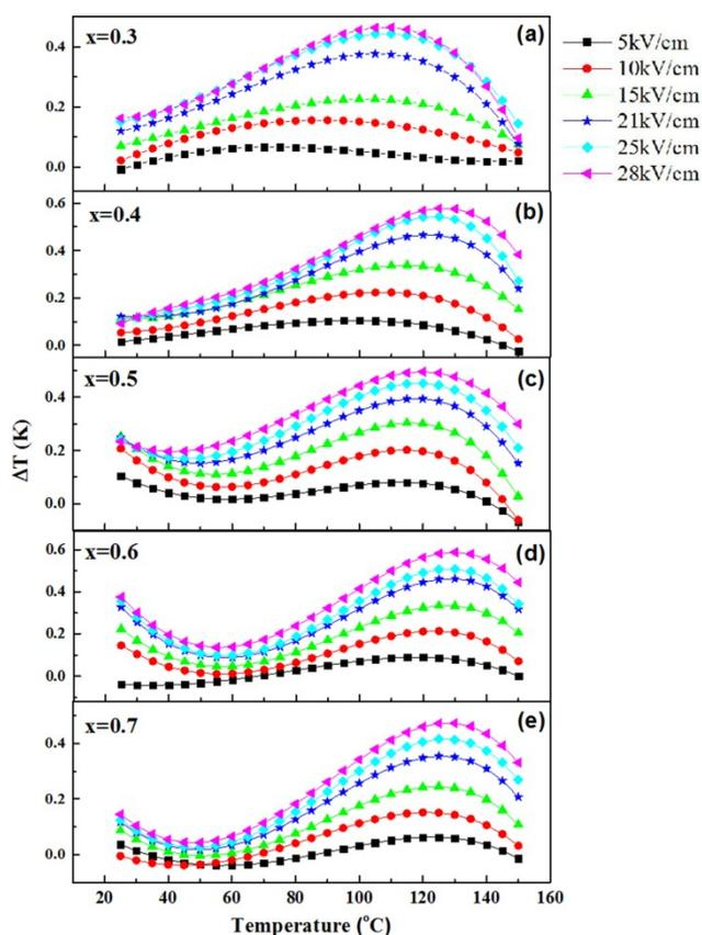
Fig.4 Electrocaloric temperature change ( $\Delta T$ ) in BZT-xBCT ceramics for (a)  $x = 0.3$ , (b)  $x = 0.4$ , (c)  $x = 0.5$ , (d)  $x = 0.6$  and (e)  $x = 0.7$  as a function of temperature and electric field.
