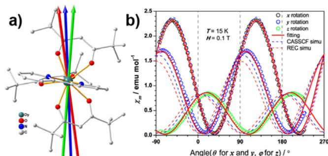
**Fig. 1** (a) View of the molecular structure of  $\text{Dy}(\text{Bu-acac})_3\text{bpy}$ . The red, blue and green arrows indicate the magnetic easy axis directions determined from experiment, CASSCF calculation and the REC model, respectively. (b) Experimental (open circles) and simulated (curves) angular dependence of the magnetic susceptibility at 15 K. Solid and dash curves represent the simulation from the best fitting of the experiment and the two theoretical results.
