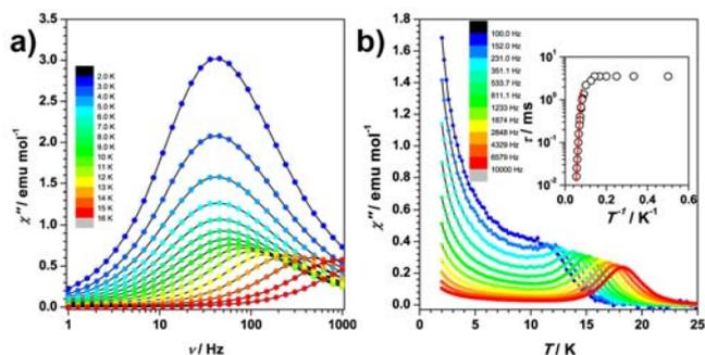
**Fig. 3** Out of phase dynamic susceptibility of magnetically pure sample at zero field as function of frequency (a) and temperature (b). Inset of (b): the relaxation time with respect to the inverse of temperature. The red line is the fitting to Arrhenius law.
