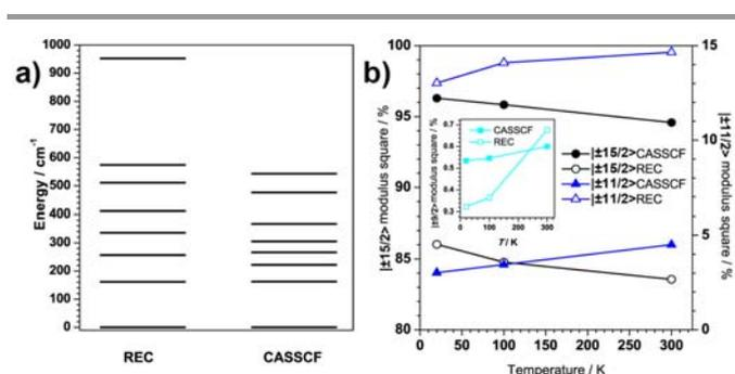
Fig. 5 (a) modulus square variation upon temperature of the dominant contributing wave functions ( $|M_J = \pm 15/2\rangle$  in circles,  $|M_J = \pm 11/2\rangle$  in triangles and  $|M_J = \pm 9/2\rangle$  in squares) to the ground state. (b) Energy levels calculated from REC model and CASSCF plot.
