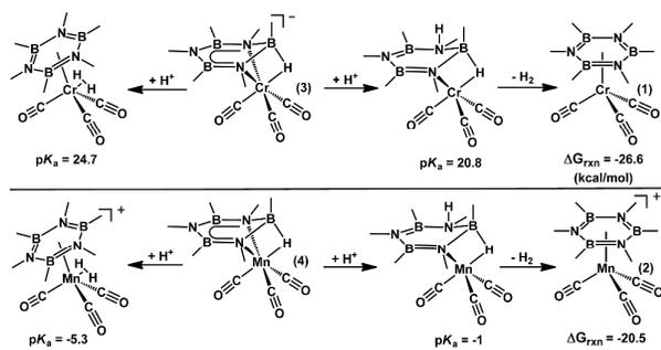
Scheme 4. Calculated  $pK_a$  values, and free energy of  $\text{H}_2$  loss, for borazine hydride adducts **3** and **4** in  $\text{Et}_2\text{O}$  solution.
