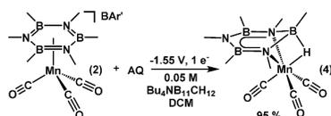
Scheme 7. Conversion of **2** to **4** by bulk electrolysis.
