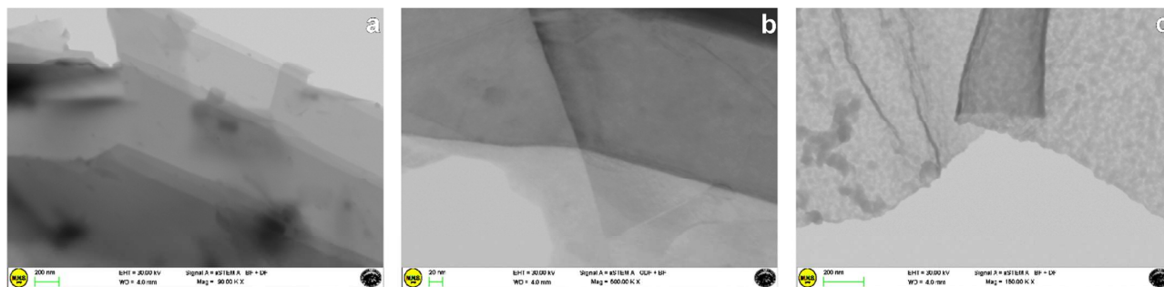
Fig. 5 STEM images of (a) graphite, (b) few layers of graphene nanosheets of G-MPO2 sample and (c) folded graphene sheet of G-MNPO sample.
