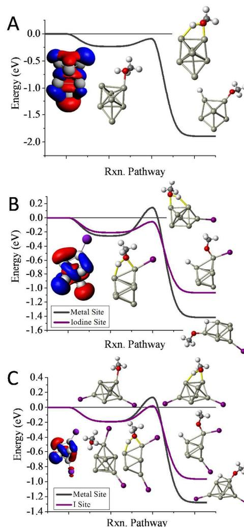
**Figure 4.** The reaction coordinates for  $\text{Al}_{7}\text{I}_{0-2}^-$  with MeOH. The calculated reaction pathways for A)  $\text{Al}_7^-$ , B)  $\text{Al}_7\text{I}^-$ , and C)  $\text{Al}_7\text{I}_2^-$  with MeOH. The red indicates the HOMO or near HOMO orbitals for degenerate orbitals, and Blue indicates LUMO or LUMO+1 orbitals that are fully unoccupied. Rxn. Pathway is abbreviated for cluster reaction coordinate and pathway.
