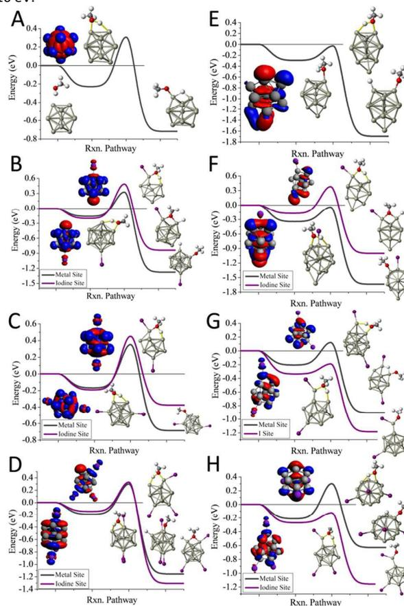
**Figure 3.** The reaction coordinates for  $Al_{13}I_{0-3}^-$  and  $Al_{14}I_{0-3}^-$ . The reaction pathways with MeOH for A)  $Al_{13}^-$ , B)  $Al_{13}I^-$ , C)  $Al_{13}I_2^-$ , D)  $Al_{13}I_3^-$ , E)  $Al_{14}^-$ , F)  $Al_{14}I^-$ , G)  $Al_{14}I_2^-$ , H)  $Al_{14}I_3^-$ . The red indicates the HOMO or near HOMO orbitals for degenerate orbitals, and Blue indicates LUMO or LUMO+1 orbitals that are fully unoccupied.
