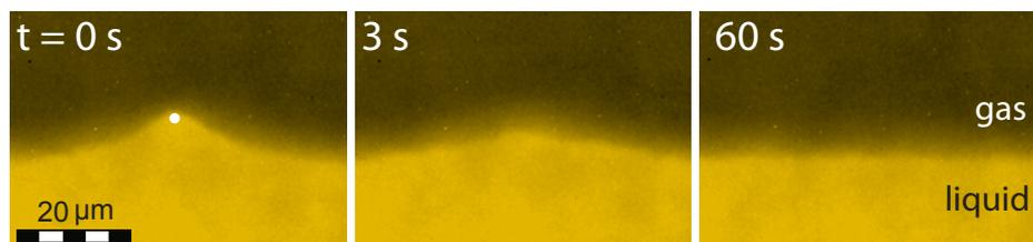
We actively control interfacial phenomena by optically trapping the interface in phase separated colloid-polymer mixtures using the gradient forces of a strongly focussed laser beam parallel to the interface.
