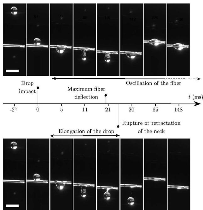
**Fig. 2** Image sequences of a drop of radius  $R = 0.76$  mm impacting a fiber ( $L = 14$  cm,  $2a = 400$   $\mu\text{m}$ ) at different velocities  $V_d$  (side view). For  $V_d = 370$   $\text{mm.s}^{-1}$  the drop is captured by the fiber (top images) whereas for  $V_d = 390$   $\text{mm.s}^{-1}$  the drop is released (bottom images). Scale bar: 2 mm.
