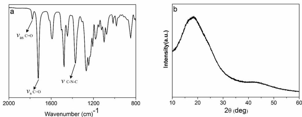
**Figure 1.** FT-IR(a) and XRD (b) spectra of TSMPI.
