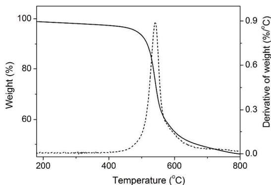
**Figure 5.** TGA spectra of the weight loss (solid line) and derivative of weight (dashed line) of TSMPI.
