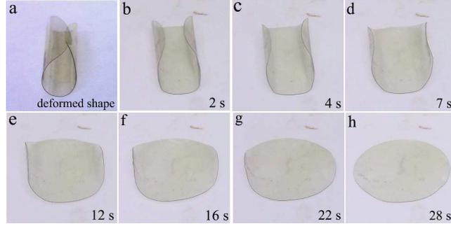
**Figure 6.** Deployable shape memory pattern of TSMPI. (a) deformed temporary shape and (b)-(h) shape recovery process of TSMPI on 190 °C hot-stage, and the subscripts indicate the time on the hot-stage.
