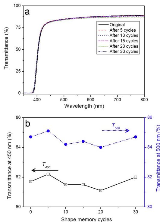
**Figure 8.** Optical properties of TSMPI exposed to shape memory cycles. (a) Transmittance before and after 5, 10, 15, 20 and 30 shape memory cycles at 350-800 nm. (b) Particular transmittance values at 450 and 500 nm after different cycles.
