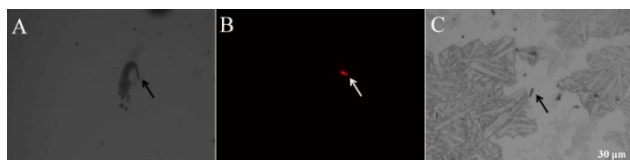
Fig. 6 (A) Microscope photo of the magnetic imprinted micromotor in seawater with target phycocyanin protein; (B) fluorescence time-lapse photo taken after the micromotor moved in seawater with phycocyanin for 20 min; (C) microscope photo of the micromotor after evaporation of the solution.
