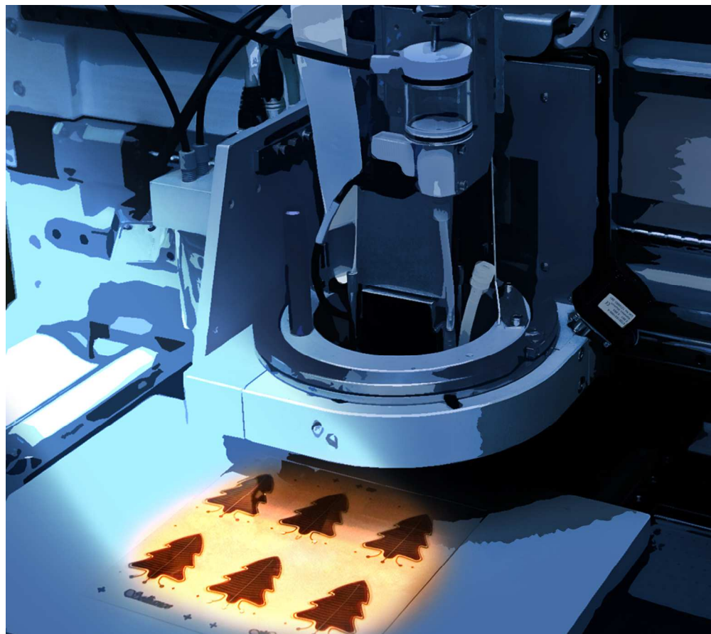
All-inkjet printed large area organic solar cells deposited from environmentally friendly solvents are demonstrated for the first time 210x186mm (300 x 300 DPI)
