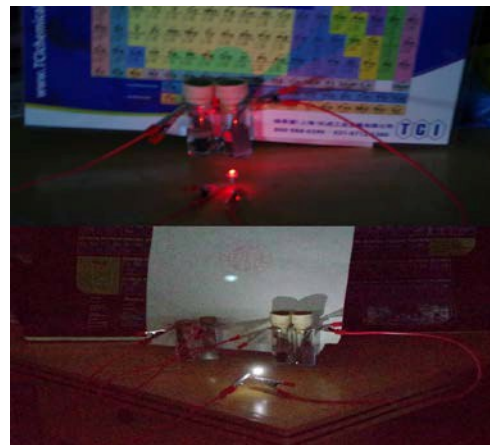
Fig. 4 LEDs powered by the assembled Zn-NiO batteries (Red, 1.7-2.3 V; White, 3-3.6 V).
