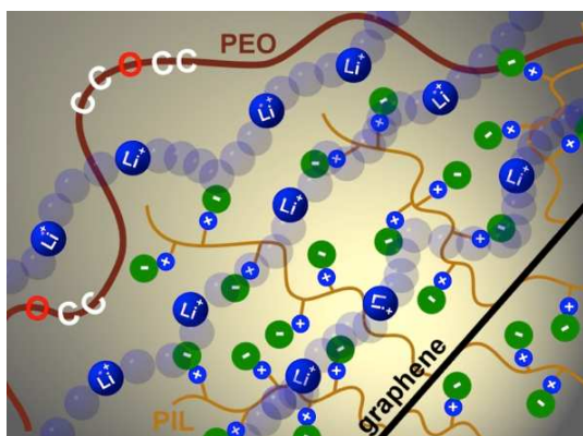
Figure 9. Illustration on Li ion transport mechanism in the PEO/ \text{Li}^+ /PIL(TFSI)-FG brush CPE.
